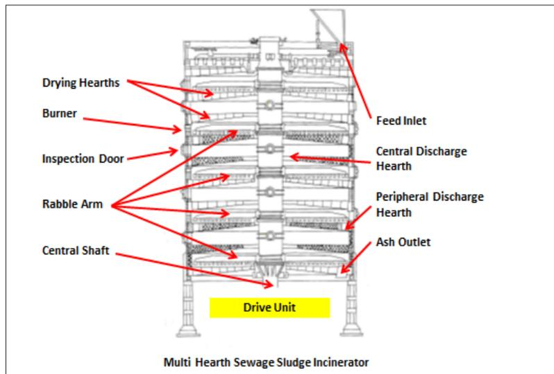
**Fig. 8 Typical multi-hearth sewage sludge incinerator**
