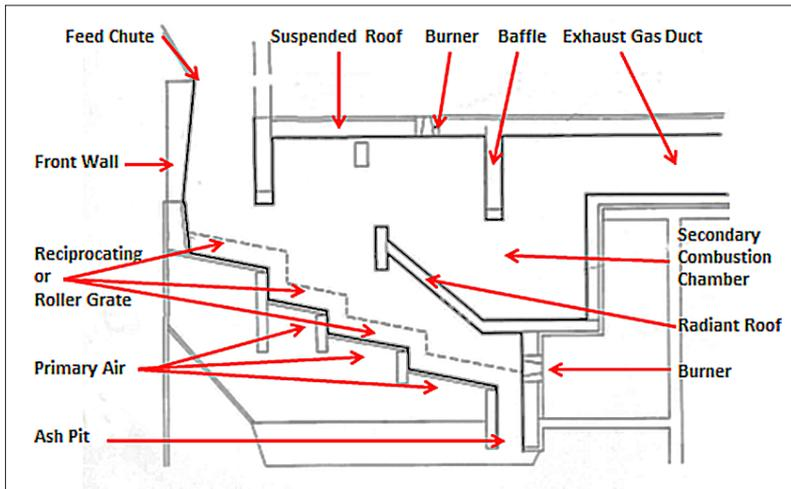
**Fig. 6** Large continuous high capacity moving grate incinerator for MSW
