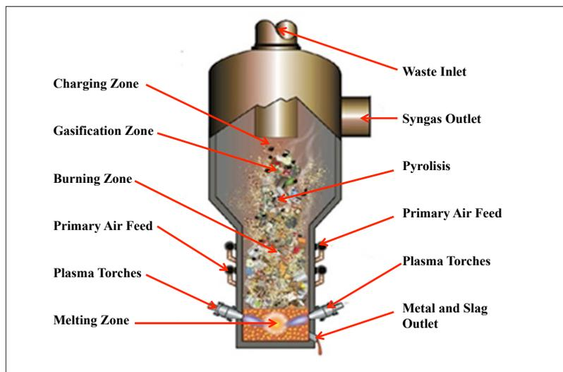
**Fig. 9 One design of a MSW plasma arc incinerator**
