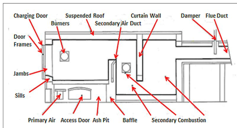
**Fig. 5** Fixed hearth batch type incinerator for MSW
