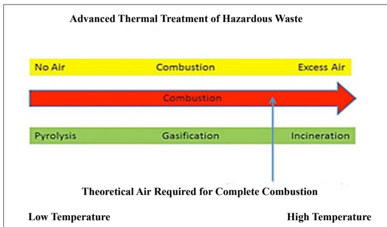
**Fig. 10** The range of thermal process types for future waste disposal
