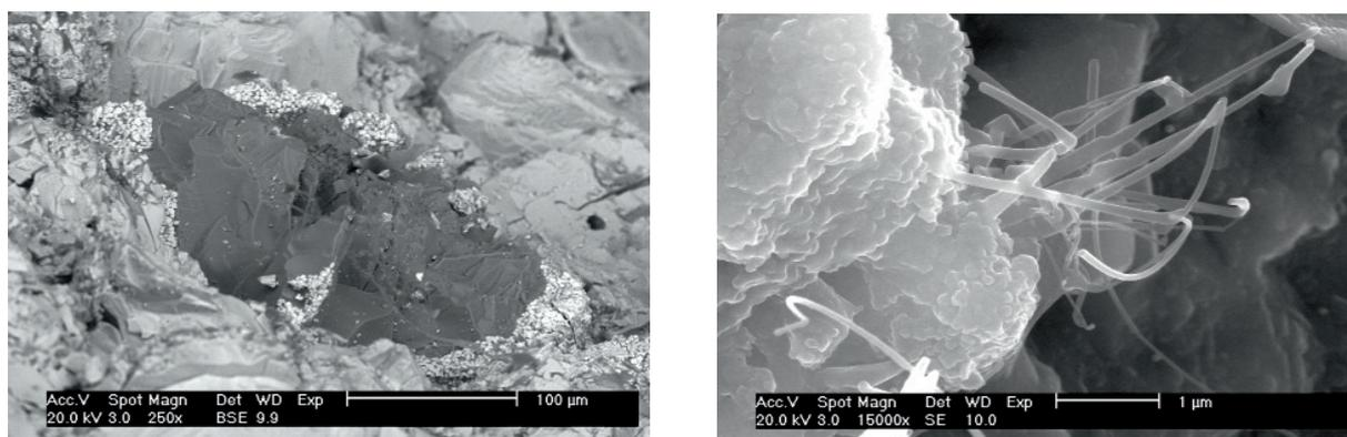
**Fig. 1** Integration of aluminium in the microstructure at 710 °C (left) and formation of AlN-whiskers at 910 °C (right)
