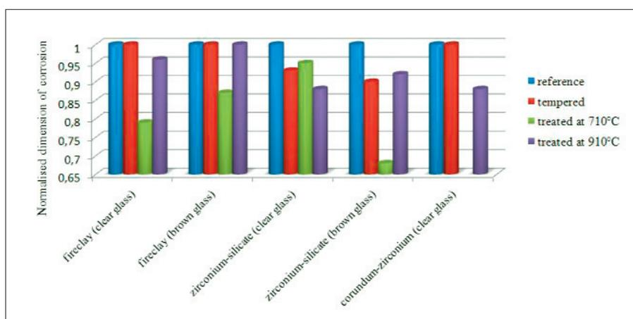
**Fig. 2** Corrosion of fireclay, zirconium-silicate and corundum-zirconium in clear and brown glass
