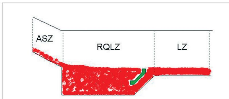
**Fig. 4** Possible construction of a segmented thin-film melter
