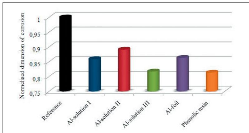
Fig. 3 Corrosion resistance of treated fireclay in clear glass after 20 h at 1400 °C
