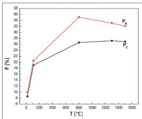
**Fig. 4** Change of apparent porosity  $P_C$  [%] of concrete C and  $P_B$  [%] of concrete B (obtained with IPP)
