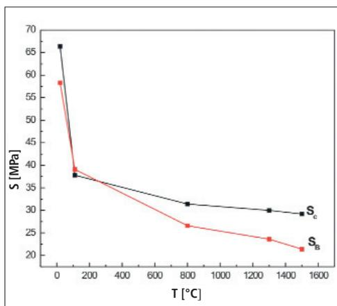
**Fig. 1** Mechanical compressive strength degradation  $S_C$  [MPa] of concrete C and  $S_B$  [MPa] of concrete B
