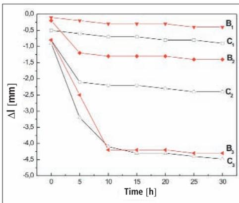
**Fig. 5** Creep deformation curves ( $\Delta l$ ) obtained during creep tests on B and C sample at three temperatures: B1 and C1 – at 1000 °C, B2 and C2 – at 1300 °C and B3 and C3 – at 1500 °C
