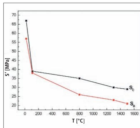
**Fig. 2** Mechanical compressive strength degradation  $S'_C$  [MPa] of concrete C and  $S'_B$  [MPa] of concrete B (calculated using UPV)
