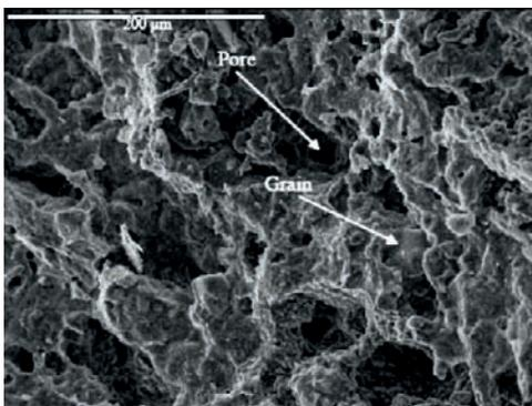
**Fig. 6** SEM of B concrete sample heat treated at 1500 °C
