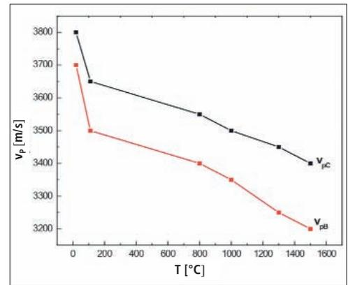
Fig. 3 Ultrasonic pulse velocity  $v_{pC}$  [m/s] of concrete C and  $v_{pB}$  [m/s] of concrete B
