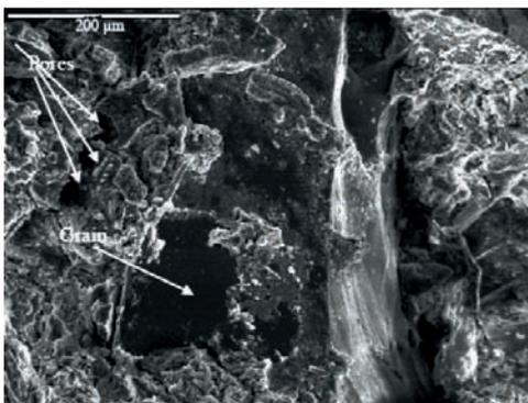
**Fig. 7** SEM of C refractory concrete heat treated at 1500 °C
