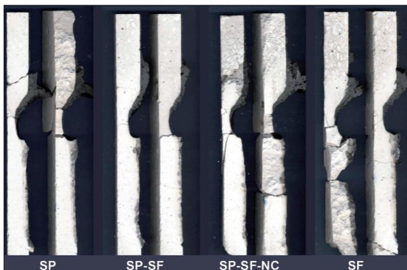
**Fig. 3** Test bars of spinel containing and spinel forming castables and mixtures thereof after induction furnace corrosion test 1650 °C/2h; C/A ratio 1,08
