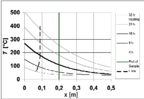
**Fig. 2** Curve of the temperature in the castable layer (drying in field practice), ( $\vartheta_a = 30\text{ }^\circ\text{C}$ ;  $L = 0,2\text{ m}$ ;  $L_{IMV} = 0,09\text{ m}$ ;  $k = 15\text{ K/h}$ ;  $a = 9 \cdot 10^{-7}\text{ m}^2/\text{s}$ )
