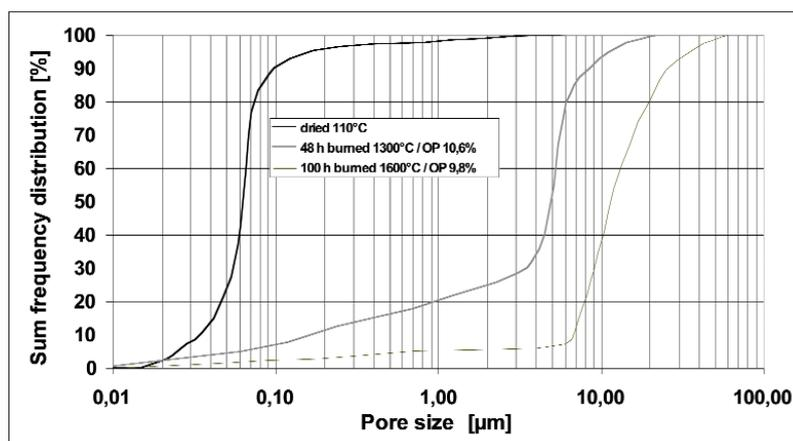
Fig. 1 Pore size distribution of an ULCC
