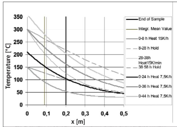
**Fig. 6** Heating and holding temperatures during drying in field practice ( $\vartheta_0 = 30\text{ °C}$ ;  $L = 0,2\text{ m}$ ;  $L_{IMV} = 0,09\text{ m}$ ;  $k = 15\text{ K/h}$ ;  $a = 9 \cdot 10^{-7}\text{ m}^2/\text{s}$ )
