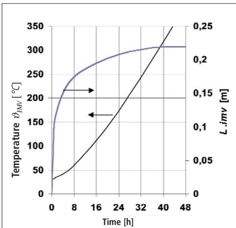
**Fig. 3** Course of the integral mean value of the temperature  $\vartheta_{IMV}$  and the location  $L_{IMV}$  as a function of time  $t$  ( $\vartheta_a = 30\text{ }^\circ\text{C}$ ;  $L = 0,5\text{ m}$ ;  $k = 15\text{ K/h}$ ;  $a = 9 \cdot 10^{-7}\text{ m}^2/\text{s}$ )
