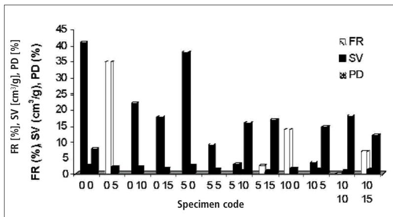
**Fig. 1** Floating ratio (FR), sedimentation volume (SV) and packing density (PD) of as-received and coated graphite powder suspensions
