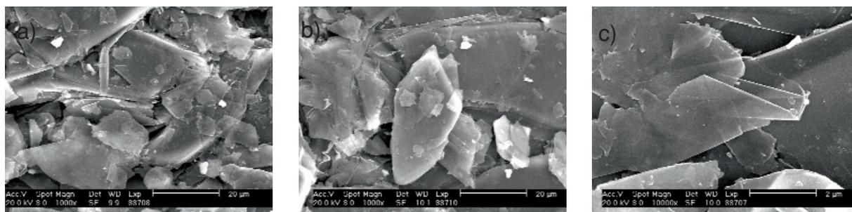
**Fig. 4** SEM photograph of raw materials and treated graphite, a) 0-0, b) 5-5, c) 10-10 specimens
