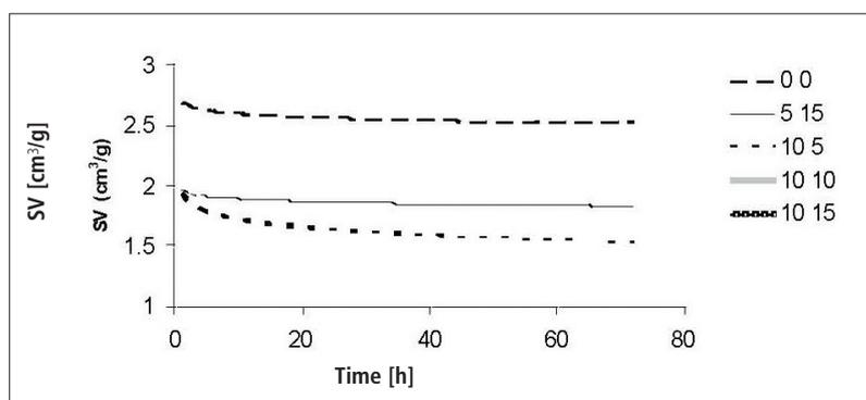
**Fig. 2** Sedimentation volume (SV) versus time of as-received and coated graphite powder suspensions
