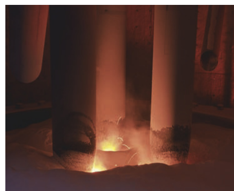
Fig. 2 Electrodes melting raw materials to make fused aluminum oxide
