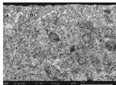
**Fig. 9** Refractory SiC mortar after salt corrosion tests at 350 °C / 500 h, overview of different zones at the hot face
