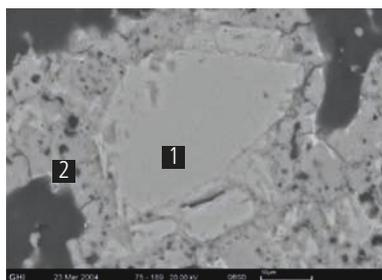
**Fig. 8** SEM micrograph of the bonding phase of nitride bonded SiC type B after 500 h oxidation resistance test at 900 °C (1 - SiC; 2 - SiO<sub>2</sub>)
