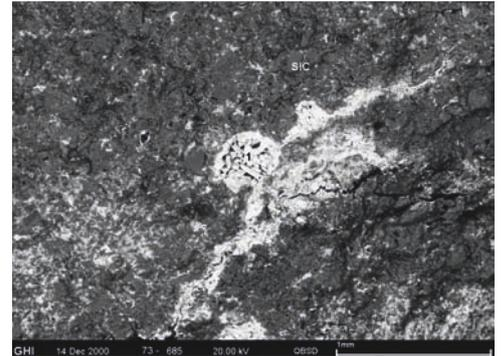
**Fig. 10 Refractory SiC mortar after salt corrosion tests at 350 °C/500 h, detail of a pore filled with salt and crack formation**
