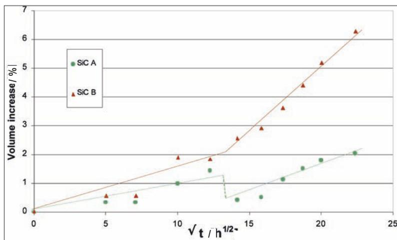
Fig. 4 Volume increase of nitride bonded SiC after oxidation resistance test at  $900\text{ }^\circ\text{C}$
