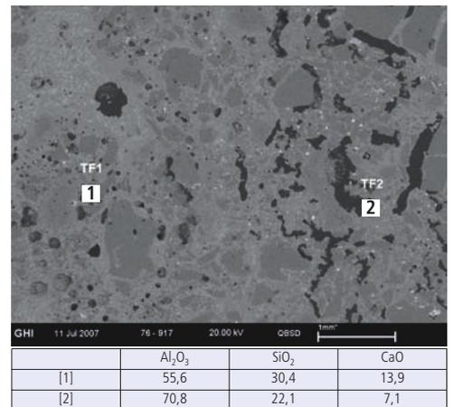
**Fig. 12 SEM micrograph: High alumina refractory with mullite bonding after slag corrosion, transition zone to porous microstructure with homogenous distribution of zircon (TF 2)**
