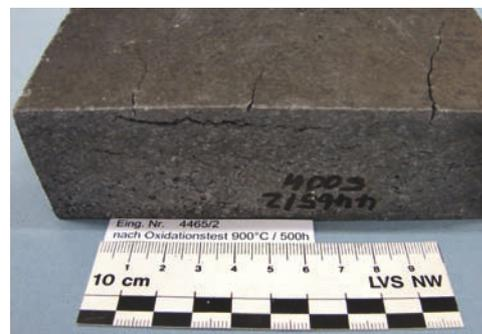
**Fig. 2 Nitride bonded SiC after laboratory oxidation resistance test at 900 °C / 500 h: Crack formation and increase of volume**
