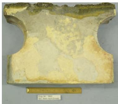
**Fig. 1 Nitride bonded SiC after operation in an industrial waste incineration plant: Slag formation at the hot face, oxidation and crack formation**
