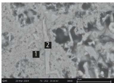
**Fig. 7** SiC Material A, detail of the bonding phase of nitride bonded silicon carbide refractory after 500 h oxidation resistance tests at 900 °C (1 – Si-O-N phase (29 % N, 38 % Si), 2 - SiC)
