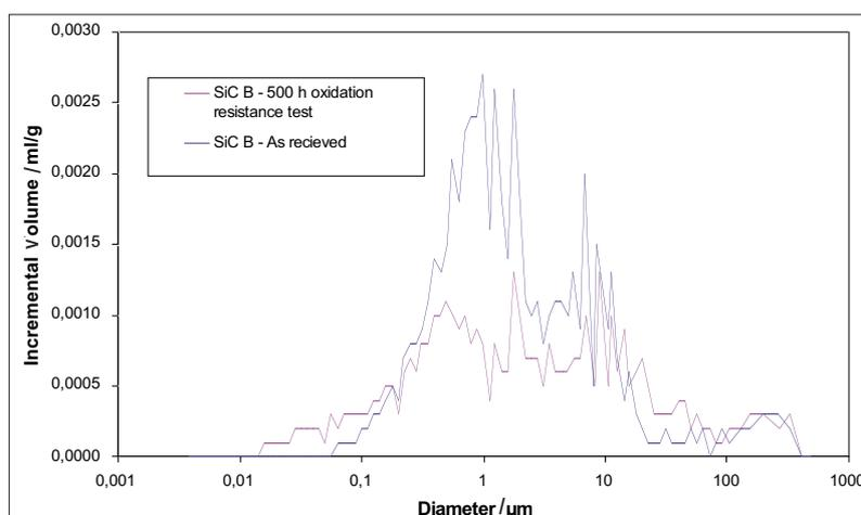
Fig. 6 Pore size distribution of SiC B before and after oxidation resistance test at  $900\text{ }^\circ\text{C} / 500\text{ h}$
