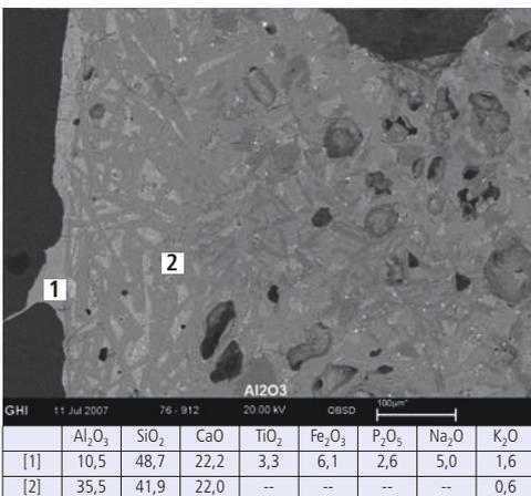
**Fig. 11 SEM micrograph: High alumina refractory with mullite bonding after slag corrosion, overview of reaction zones at the hot face**
