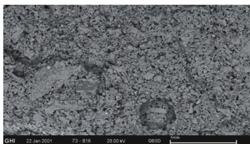
**Fig. 3 SEM micrograph of SiC mortar as received**
