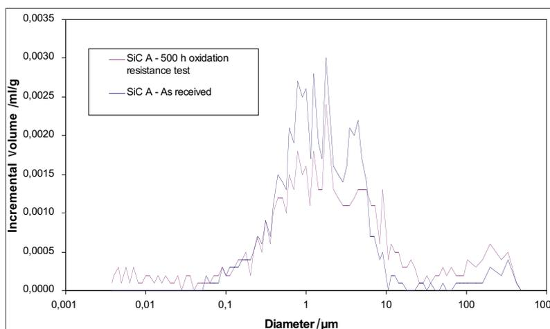
Fig. 5 Pore size distribution of SiC A before and after oxidation resistance test at  $900\text{ }^\circ\text{C} / 500\text{ h}$
