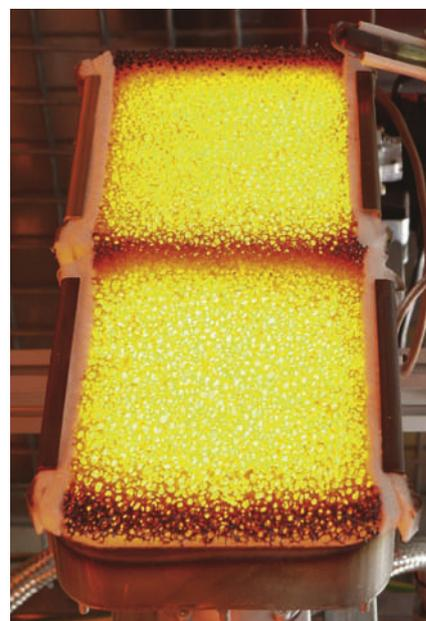
Fig. 2 Square porous burner
