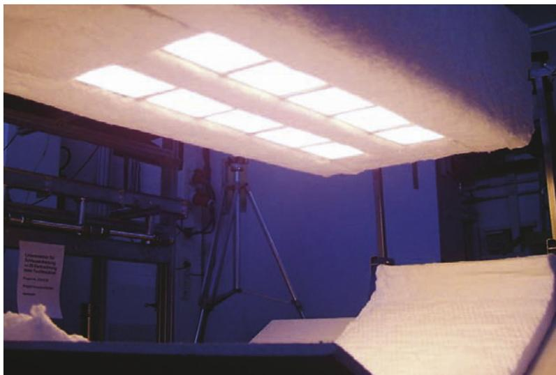
Fig. 3 Porous burner for glass heating consisting of different and separately regulable sections
