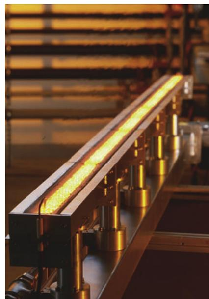
Fig. 1 Line porous burner
