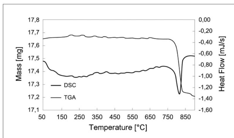
**Fig. 2** DSC/TGA for xonotlite; the mass loss and the endothermic peak around  $815\text{ }^{\circ}\text{C}$  are related to the hydroxyls decomposition and the simultaneous recrystallization to the low temperature wollastonite polymorph [22]
