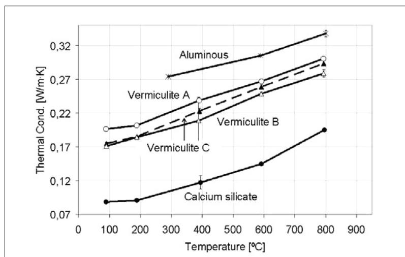
**Fig. 4** Thermal conductivity of thermal insulating materials [31]
