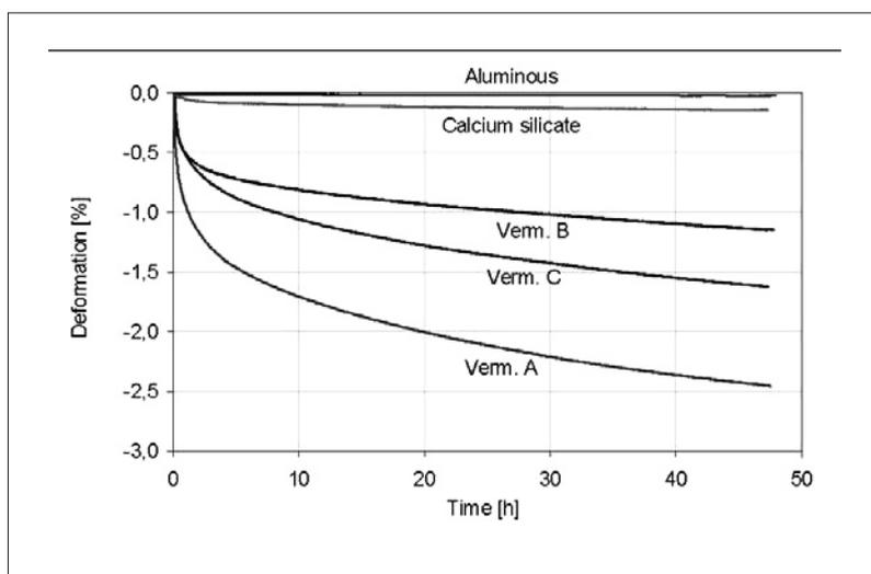
**Fig. 6** Creep curves for vermiculite (producers A, B and C), calcium silicate and aluminous insulating materials [31]
