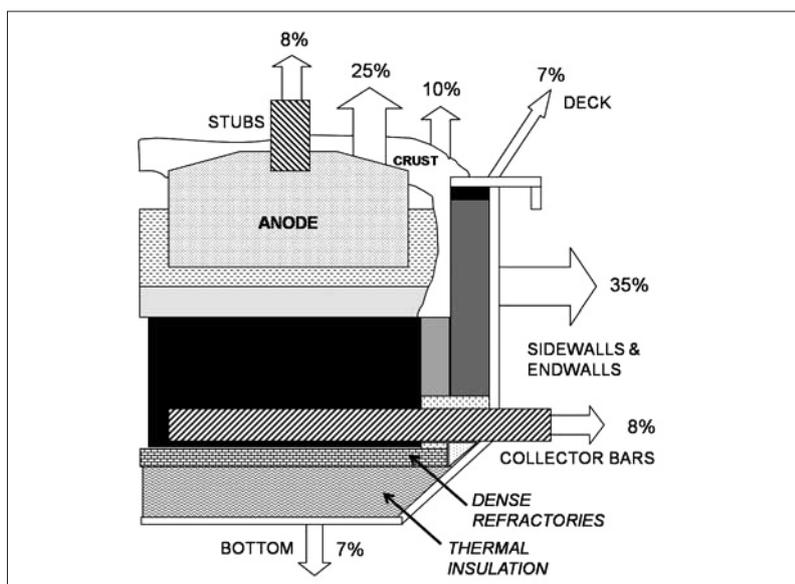
**Fig. 1** Average heat losses from an aluminium cell [16]
