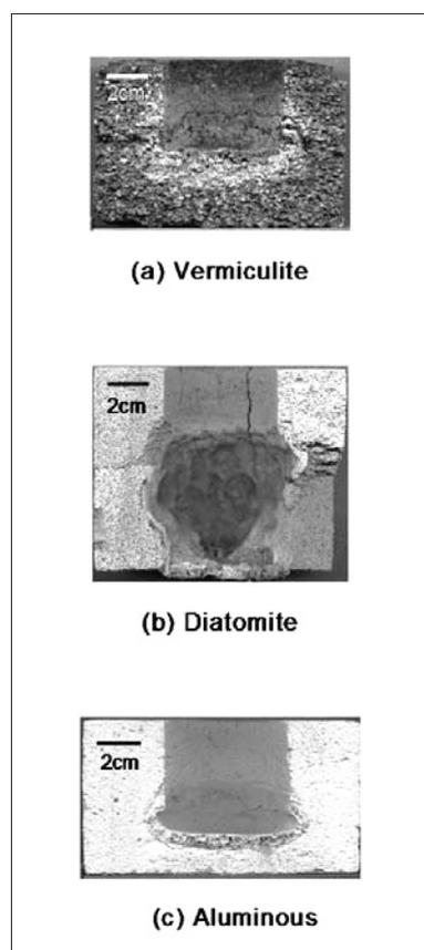
**Fig. 3** Bath attack on vermiculite, diatomite and aluminous insulating materials [26]
