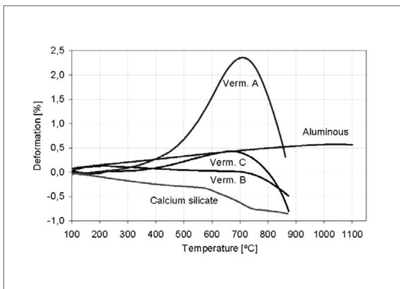
**Fig. 5** Refractoriness under load curves (0,02 MPa) for vermiculite (producers A, B and C), calcium silicate and aluminous insulating materials [31]
