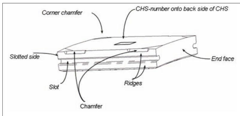
Fig. 3 Ceramic heat shield
