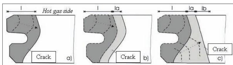
**Fig. 7** Thermally and thermomechanically induced macro cracks in ceramic heat shields. Crack growth is shown in a cross-sectional view with cracks originating from the edges of the heat shield with the slot
