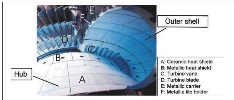
Fig. 2 View into an annular combustor (viewed in direction of flow)
