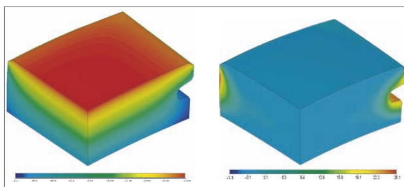
**Fig. 6** Temperature and stress distribution under steady-state conditions; each view shows one quarter of a heat shield
