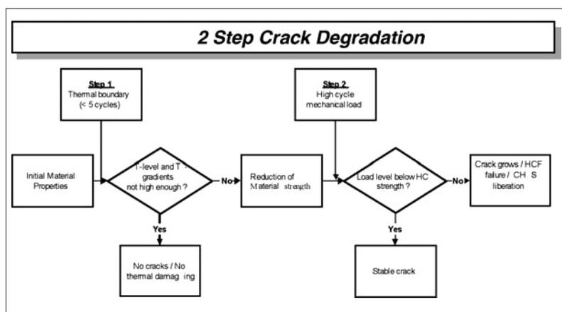
**Fig. 8** Crack growth in ceramic heat shields
