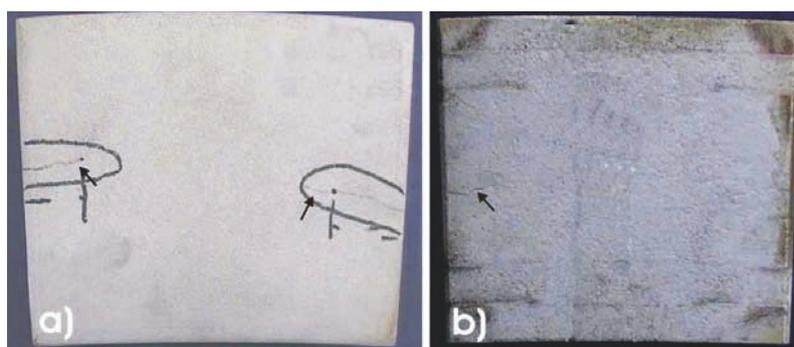
**Fig. 5** Crack types in ceramic heat shields in service, a) Circumferential crack on combustor side (hot side) b) Circumferential crack on back side (cold side)
