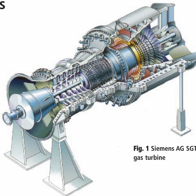
Fig. 1 Siemens AG SGTX-4000F gas turbine
