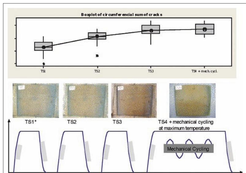
**Fig. 11 Crack formation as a function of loading in the thermal fatigue test facility; a typical test consists of three thermal shocks followed by a final fourth thermal shock during which the heat shield is cycled mechanically during the hold time at maximum temperature**
