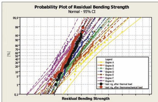
**Fig. 13** Comparison between results from thermal fatigue test facility and ceramic heat shields subjected to plant operational loadings
