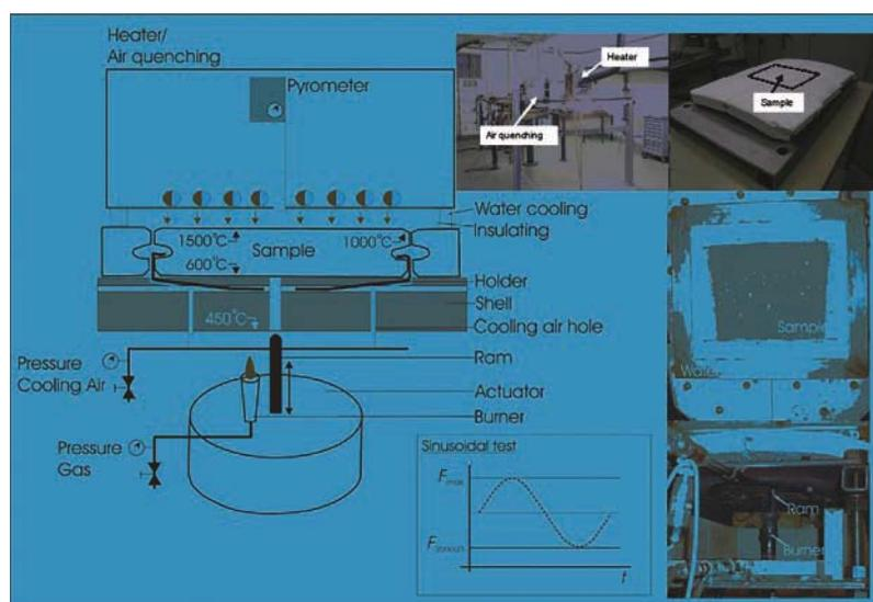
Fig. 9 Schematic setup of thermal fatigue test facility
