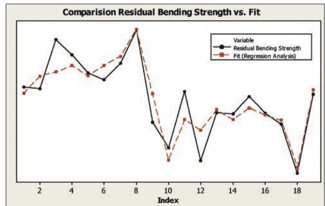
**Fig. 14** Comparison between residual bending strength of ceramic heat shields taken from a plant with calculated values ( $r^2$  from regression analysis  $> 80\%$ ) yielded by nondestructive examination (crack length and eigenfrequency)
