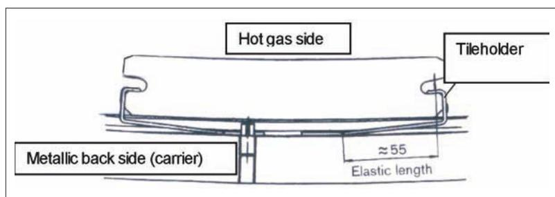
Fig. 4 Heat shield with holders
