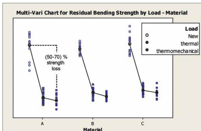
**Fig. 12 Load-dependent residual strength levels [MPa] for ceramic heat shields in the thermal fatigue test facility**
