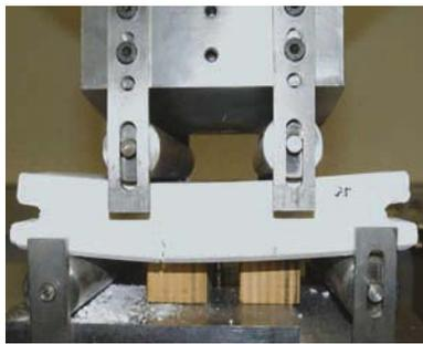
**Fig. 10 Four-point bending test on entire heat shield (hot side under tensile stress)**
