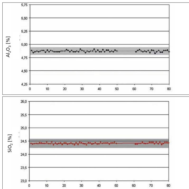
**Fig. 4 Precision trial for Al<sub>2</sub>O<sub>3</sub> and SiO<sub>2</sub> for a raw material**
