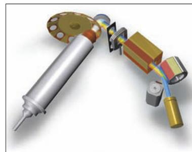
**Fig. 3 Analytical flexibility: Instrumental setup of sequential wavelength dispersive X-ray fluorescence spectrometers**
