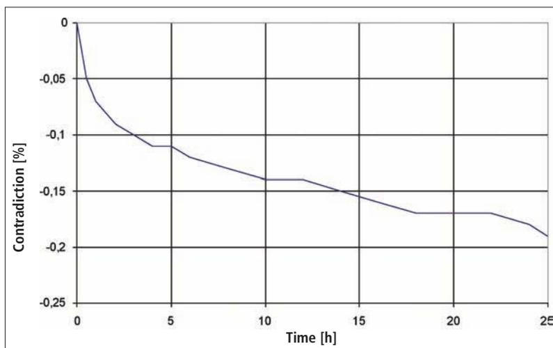
**Fig. 12** Creep in compression according to DIN EN 993-9, Brick CL at 1280 °C / 25 h / 0,2 MPa
