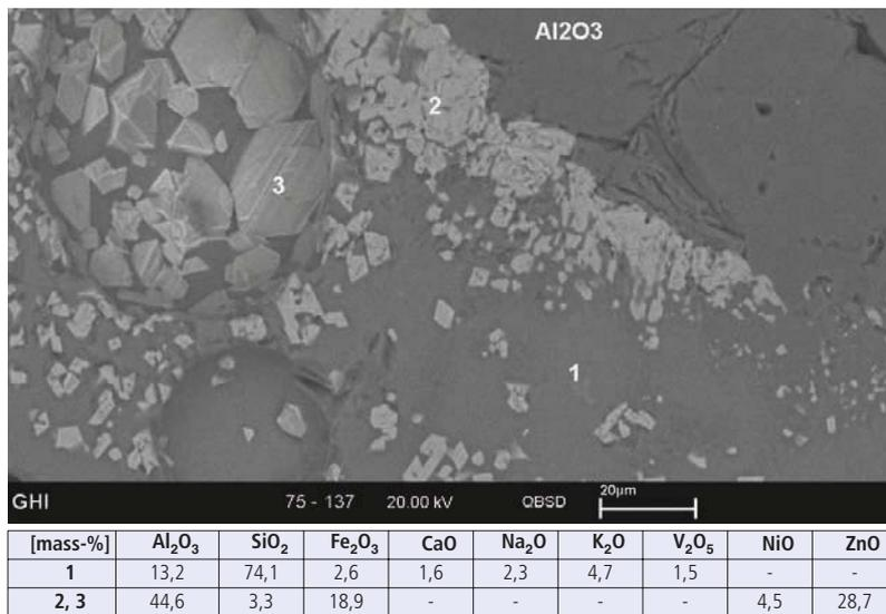
**Fig. 11** SEM micrograph, OP after operation, transition of infiltration zone to refractory, hot face
