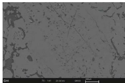
Fig. 5 Brick OP as received for use in open top anode baking furnace
