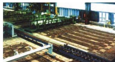
Fig. 2 Open top ring pit furnace for anode baking [1]
