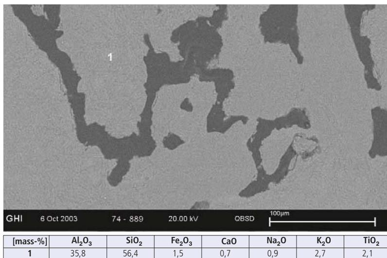
**Fig. 8** SEM micrograph, brick CL after operation, porous matrix cold face
