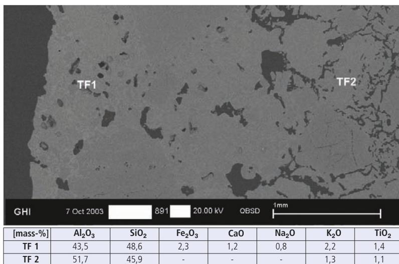
**Fig. 6** SEM micrograph, brick CL after operation, overview hot face
