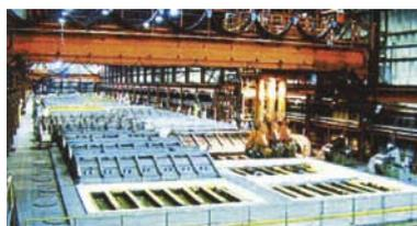
Fig. 1 Closed ring pit furnace for anode baking [1]
