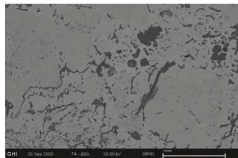
Fig. 4 Brick CL as received for use in closed anode baking furnace
