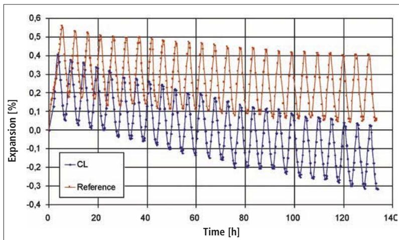
**Fig. 13** Creep in compression 1280 °C – 800 °C – 1280 °C, load 0,2 MPa, brick CL and reference material
