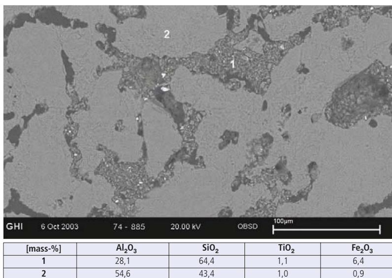
**Fig. 7** SEM micrograph, brick CL after operation, matrix near hot face
