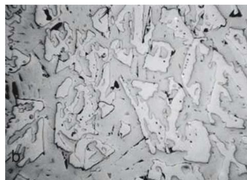
**Fig. 2 a) Monofrax H fused cast  $\beta$ -alumina refractory ( $\beta \sim Na_2O \cdot 9,2 Al_2O_3$ ) and b) Monofrax M fused cast  $\alpha/\beta$ -alumina refractory ( $\alpha = Al_2O_3$  and  $\beta \sim Na_2O \cdot 8,2 Al_2O_3$ )**
