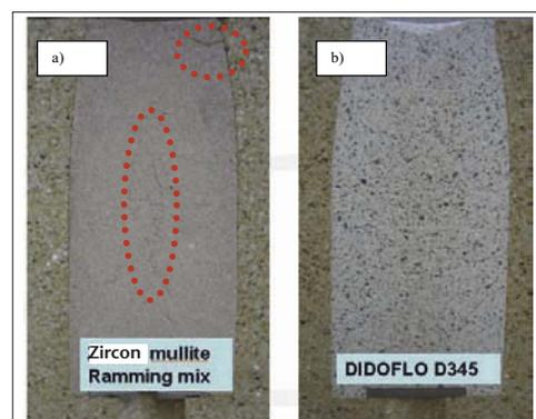
**Fig. 4 a) The stud hole filled with ramming mix based on zircon mullite, after firing at 1100 °C: cracks formed b) The stud holes filled with DIDOFLO D345, after firing at 1100 °C: no cracks or open joints**
