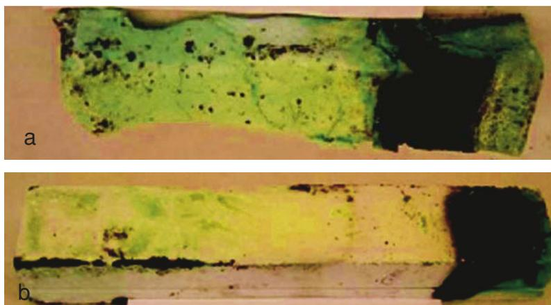
Fig. 1 a) Standard silica grade and b) STELLA GNL after 3 months in an oxy-fuel furnace
