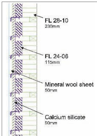
**Fig. 11** Side-wall lining with lightweight insulating bricks
