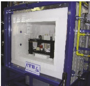
**Fig. 7 Chamber kiln of CTB Berlin used to fire cordierite ceramic**
