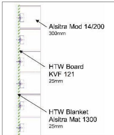
**Fig. 10** Side wall lining with Alsitra modules
