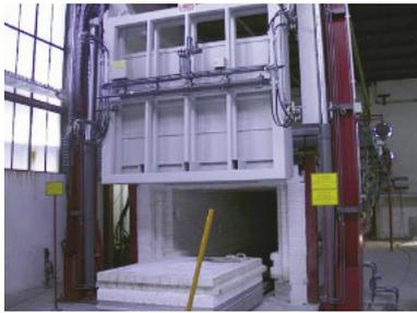
**Fig. 5 Shuttle kiln 1600 °C (Laeis)**
