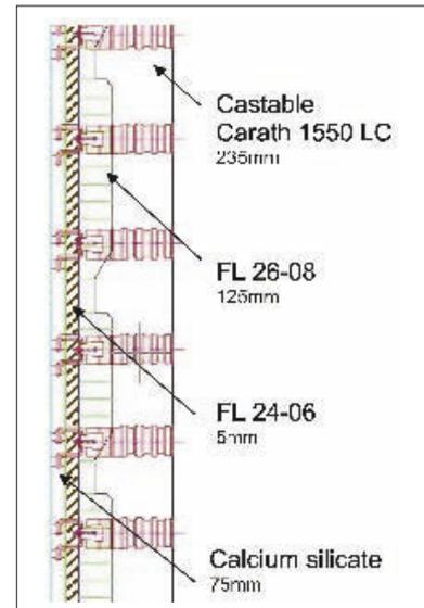
**Fig. 12** Side-wall lining with refractory castable
