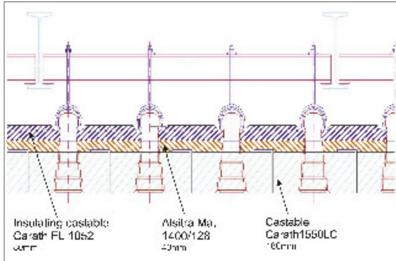
Fig. 2 Schematic diagram of refractory castable-prefabricated roof
