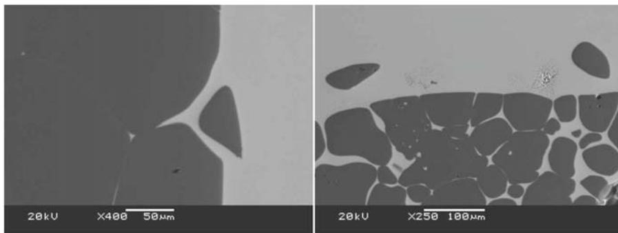
**Fig. 7** Backscatter electron images at the phase boundary of the bottom part of sintered MgO
