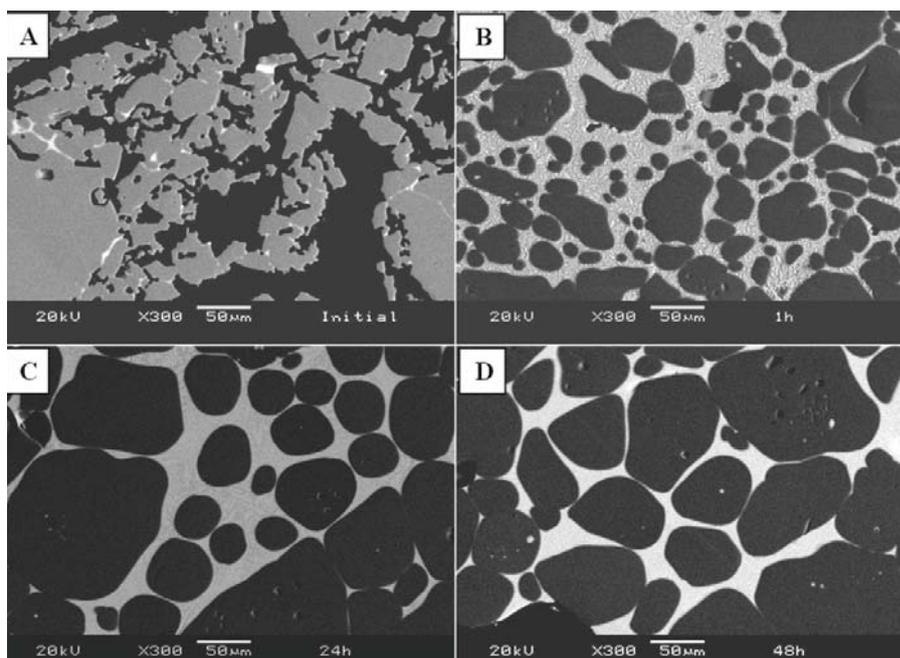
Fig. 4 Backscatter electron images of microstructural transformation of MgO through particle disintegration and Ostwald-ripening, A = 3 h at 1650 °C, no slag = pre-treatment for B, C, D, B = 1 h / C = 24 h / D = 48 h in contact with MgO saturated slag at 1600 °C, 300-fold magnification
