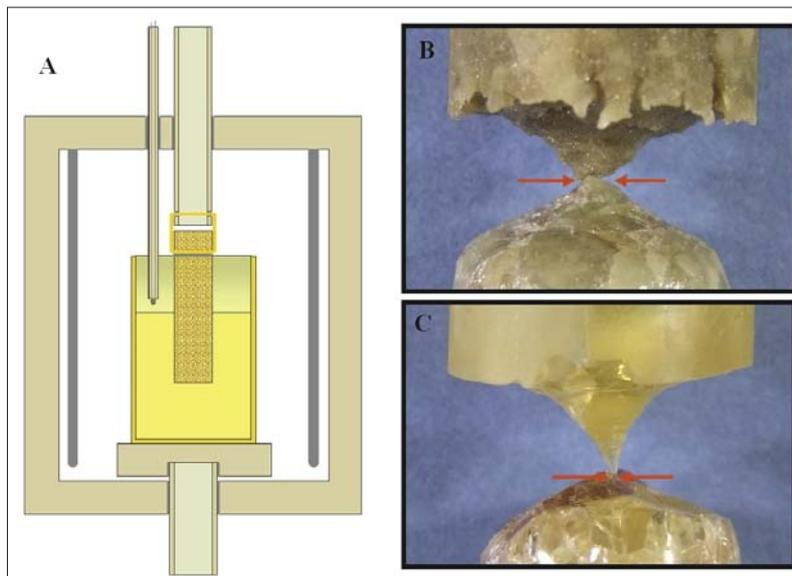
**Fig. 5** Schematic experimental setup (A) and macroscopic appearance of specimens after the test at the three phase line, B = sintered MgO ( $\epsilon = 0,133$ ), C = fused MgO ( $\epsilon = 0$ )
