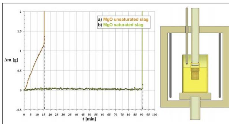
Fig. 3 Time dependent mass change  $\Delta m$  (left) and schematic experimental setup (right)
