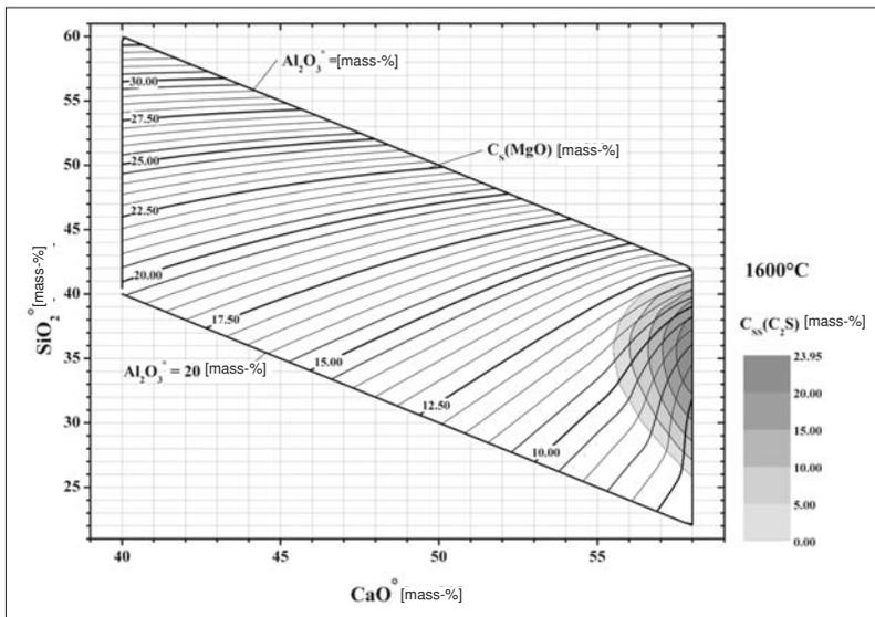
**Fig. 2**  $C_S(\text{MgO})$  at 1600 °C for lime-silicate slag, grey-staged shading = range of MgO/ $C_2S$  saturation [1, 11]
