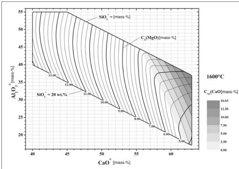
**Fig. 1**  $C_S(\text{MgO})$  at 1600 °C for lime-aluminate slag, grey-staged shading = range of MgO/CaO saturation [1, 11]
