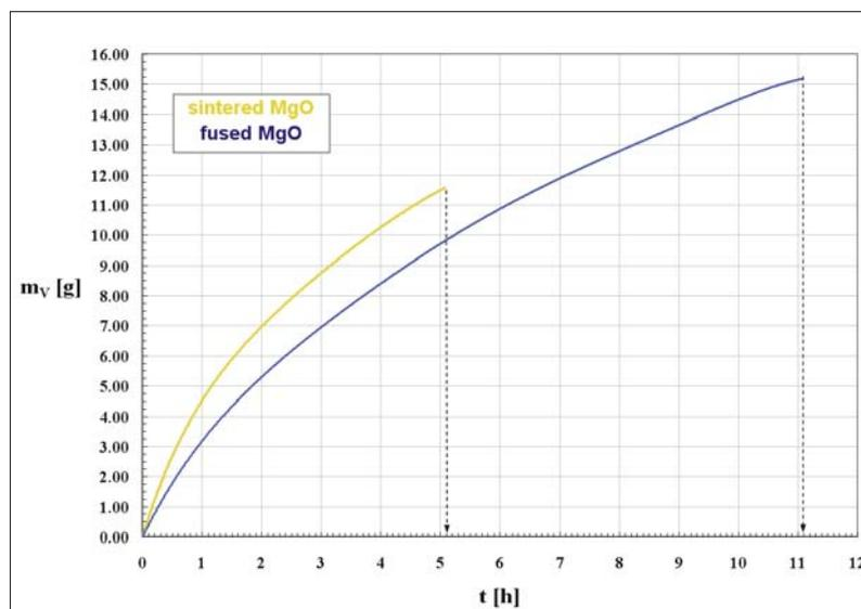
**Fig. 6** Time dependent development of actual slagged mass  $m_v$  with indication of the moment of cut through
