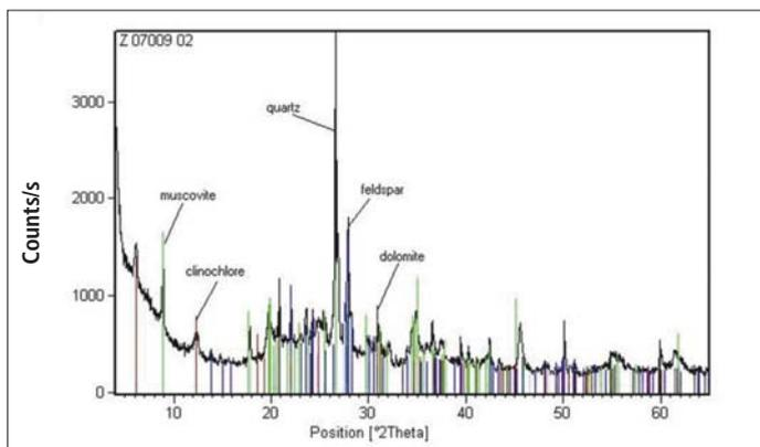
Fig. 3 XRD pattern of clayey diatomite from Drymos
