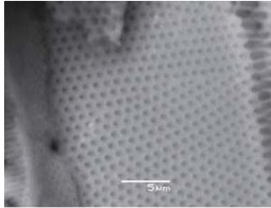
**Fig. 14** Florina-Kleidi sample, fired at 650 °C; similarly to Drymos, its biogenic silica dissolution is negligible, the diatom frustules persist
