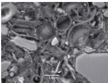
**Fig. 11** Drymos sample, calcined at 750 °C; no intense dissolution, the diatom frustules are preserved
