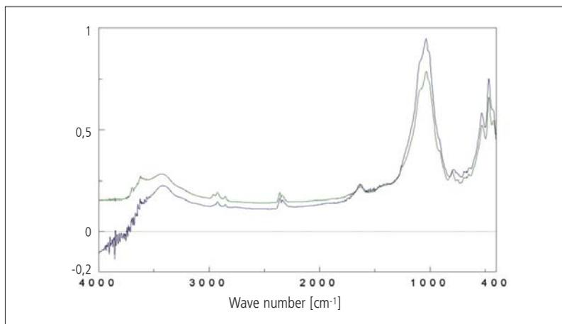
**Fig. 9** IR spectroscopy for raw materials Drymos – green line; Florina-Kleidi – blue line
