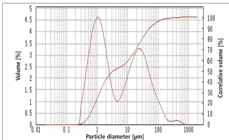
Fig. 1 Particle size distribution of the fly ash
