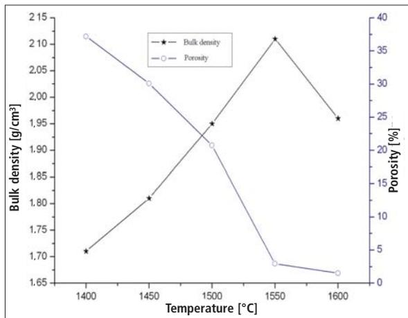
**Fig. 2** Volume density and porosity of the sintered specimens
