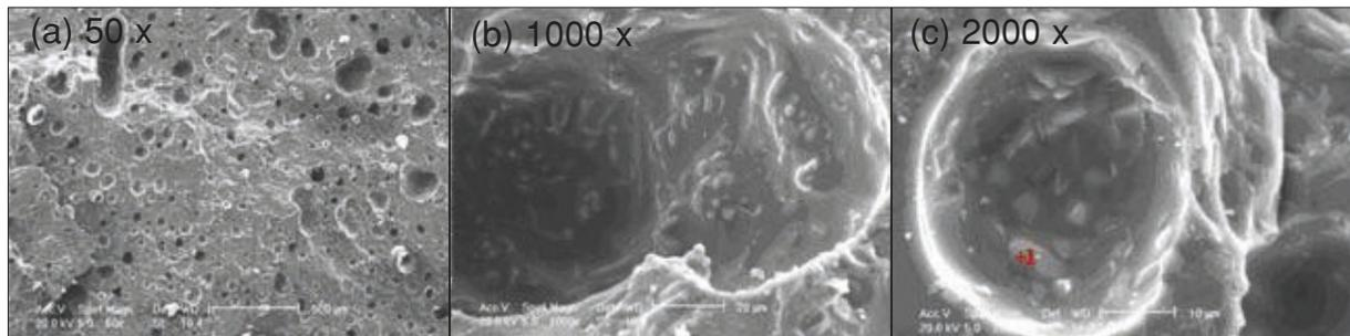
**Fig. 4** SEM micrographs of specimens sintered at 1600 °C / 3 h; a) 50x, b) 1000x, c) 2000x
