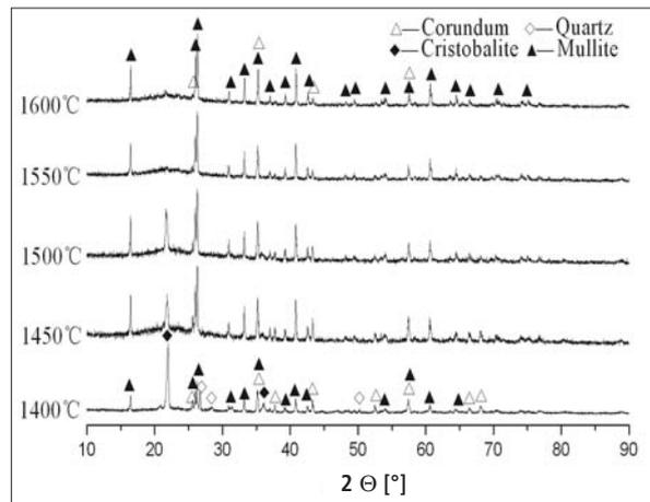
**Fig. 3** XRD patterns of sintered specimens
