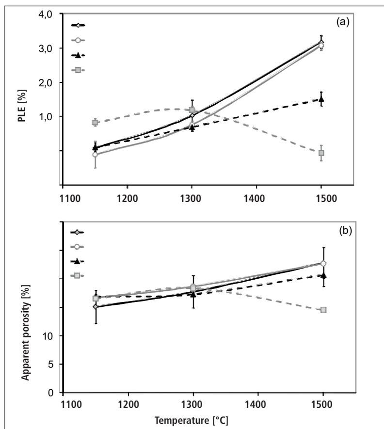
**Fig. 1** a) Permanent linear expansion (PLE) and b) apparent porosity as a function of the firing temperature
