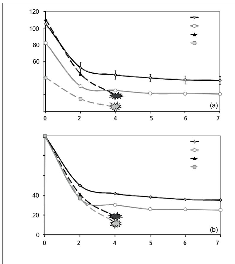
**Fig. 3** Thermal shock evaluation ( $T = 1000\text{ °C}$ ) as a function of the number of cycles, for castables previously fired at 1500 °C for 5 h, presented as a) E absolute values, and b) E normalized values
