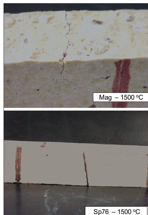
**Fig. 4** Fractures detected during the thermal shock cycling for the compositions Mag and Sp76
