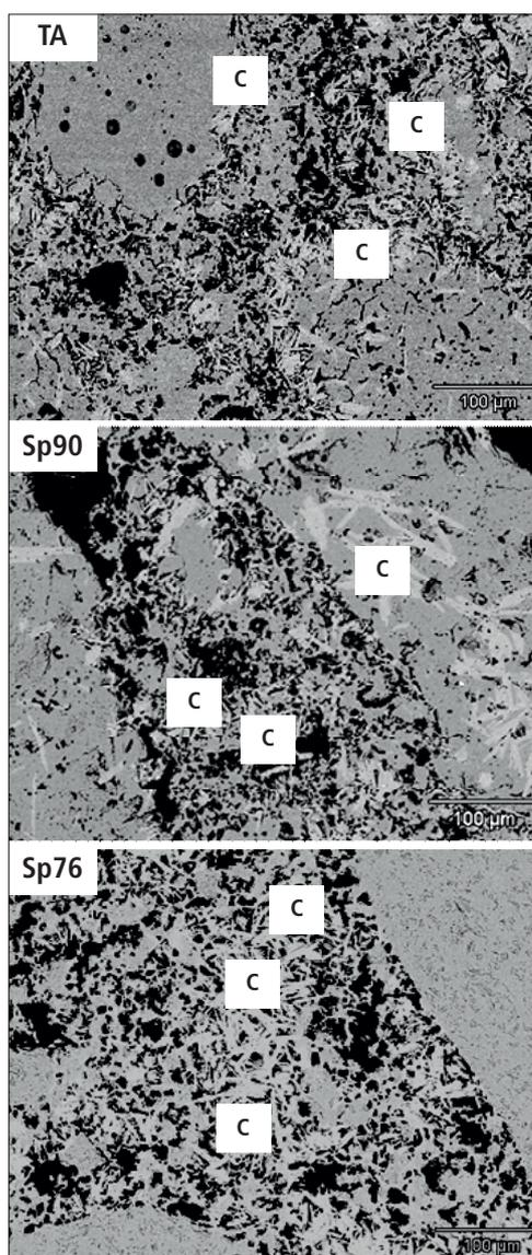
**Fig. 5** Castable microstructures of the  $CA_6$ -containing (C) compositions (TA, Sp90 or Sp76), pointing out this phase distribution, after firing at 1500 °C for 5 h
