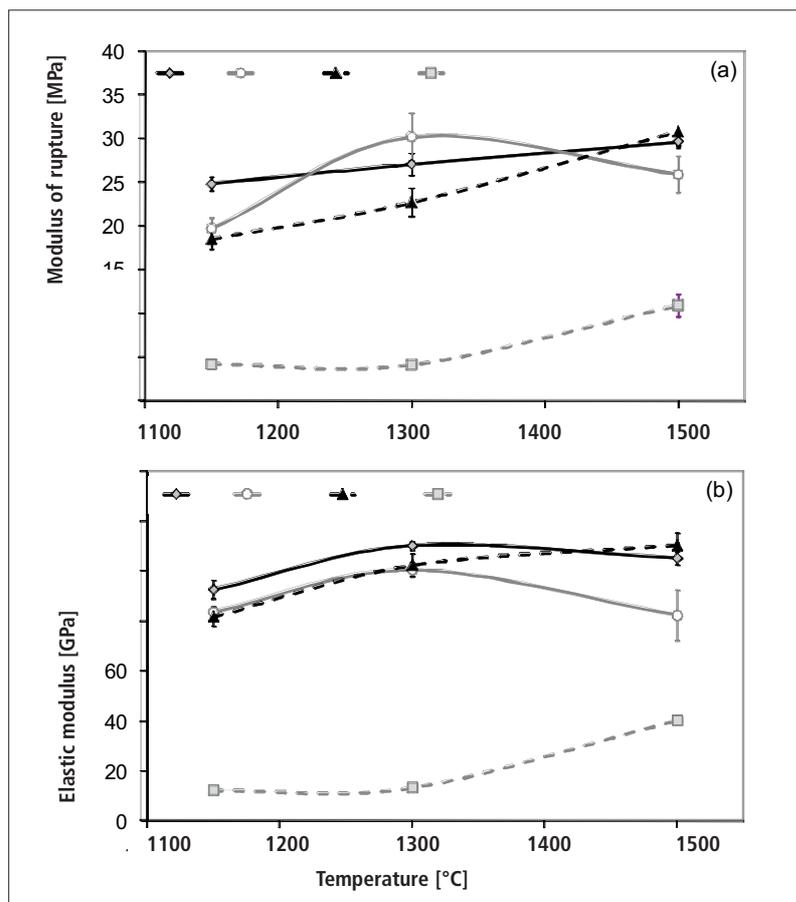
**Fig. 2a** Modulus of rupture and **b)** elastic modulus as a function of the firing temperature
