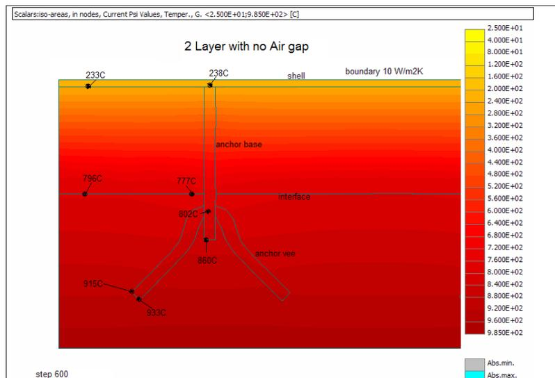
Fig. 4 2D heat transfer analysis showing the temperature profile around the anchor (no air gap at interface)
