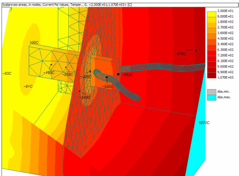
**Fig. 9** 3D temperature profile for a two layer system with high convection the shell (100W/m<sup>2</sup> · K)
