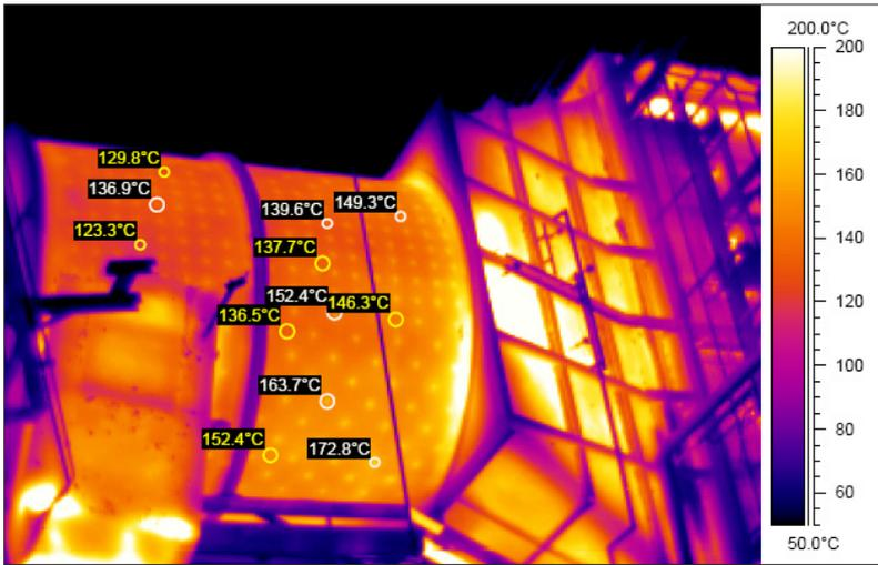
**Fig. 1** Thermovision of furnace shell showing anchor base hot spots (white circles)
