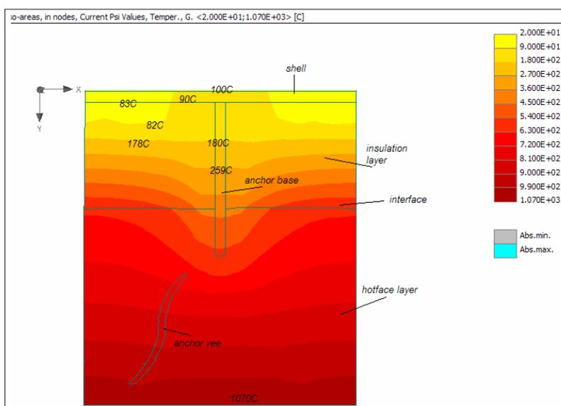
Fig. 10 Elevation view showing the temperature profile near the centre of the anchor
