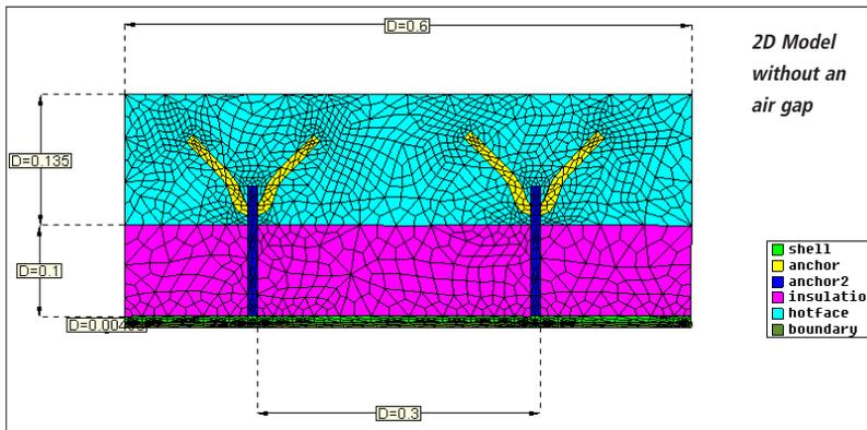
**Fig. 2** Geometry for 2D thermal analysis showing anchors and refractory layers
