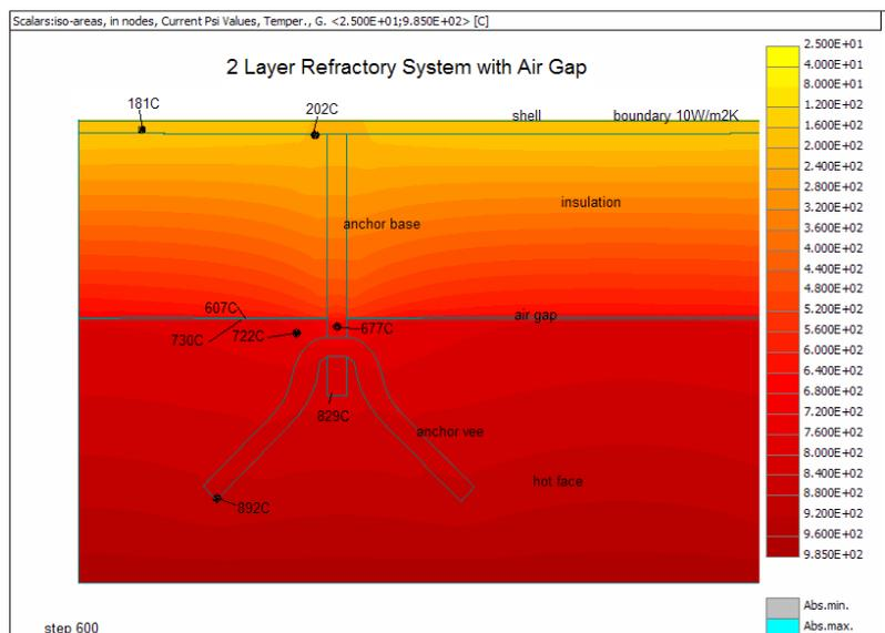
Fig. 6 2D thermal model (1/2 section) with an air gap at the interface between the concrete layers, shell boundary convection of 20 W/m<sup>2</sup> · K
