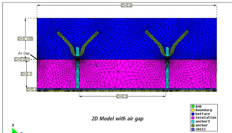
Fig. 5 2D two layer concrete model with an air gap
