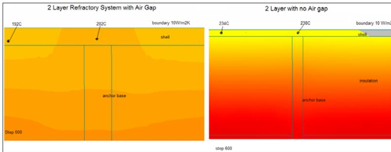
**Fig. 7** Overlay of anchor base and shell hot zones showing increased temperature area
