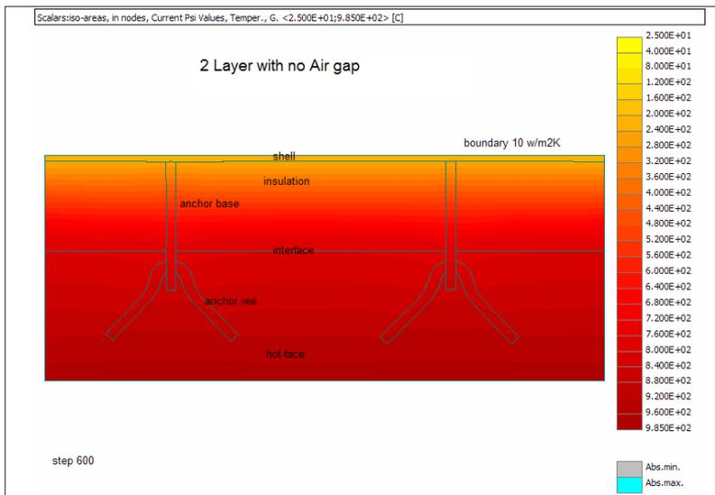
**Fig. 3** 2D two layer thermal model with refractory anchors showing the overall temperature profile and temperature bridging between the anchor vees
