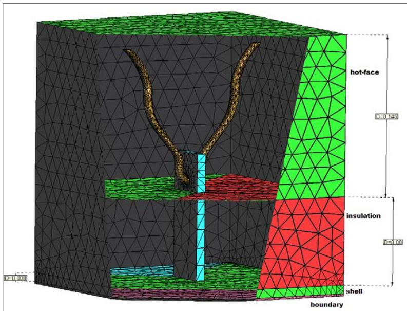
**Fig. 8** 3D model of a two layer refractory system with cut-out showing anchor profile
