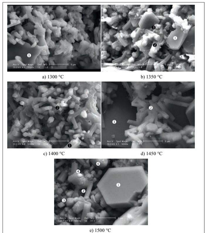
**Fig. 5** SEM images of specimens B under different nitriding temperatures: 1 – corundum, 2 – SiAlON, 3 – MgAl<sub>2</sub>O<sub>4</sub>, 4 – fused drop
