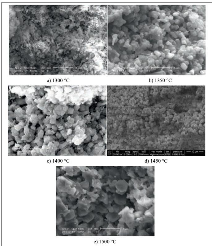
**Fig. 4** SEM images of specimen A at different nitriding temperatures
