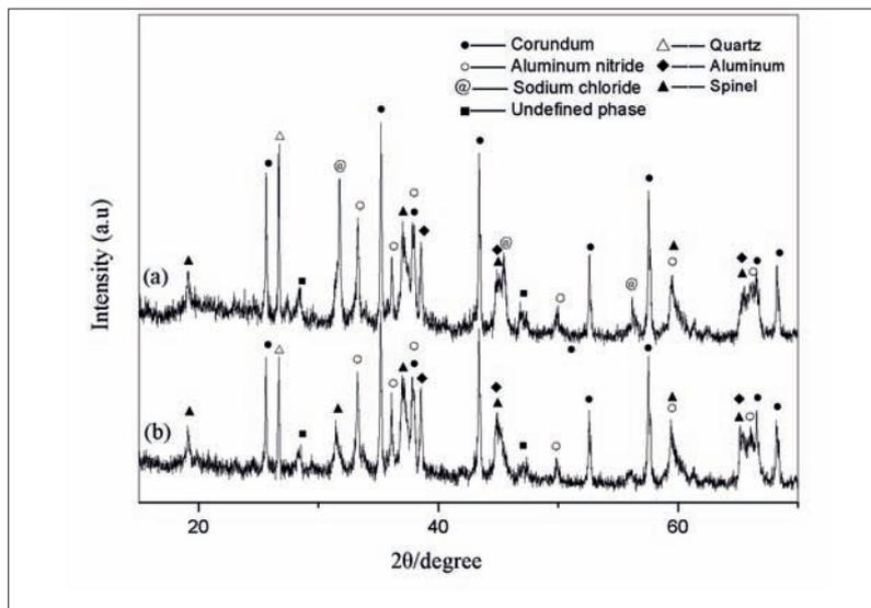
**Fig. 1** X-ray diffraction patterns: a) aluminium dross; b) water-treated aluminium dross
