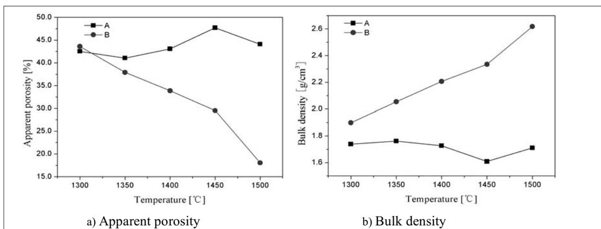
**Fig. 2** Apparent porosity and bulk density of specimens at different nitriding temperatures
