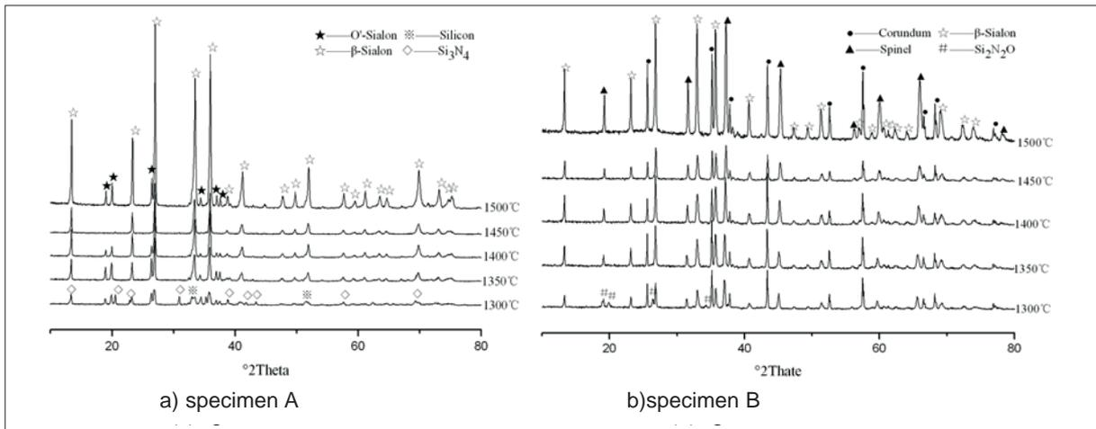
**Fig. 3. XRD patterns of specimens at different nitriding temperature**
