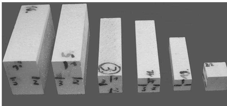
Fig. 1 Test specimens used in [2], from left: Australian bar, EN shape A, EN shape B, US bar (normally for MOR only), Indian/Japanese bar, US cube (for CCS only)
