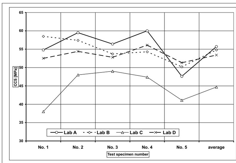
Fig. 4 Comparison of drilled cylinders CCS measured in different laboratories
