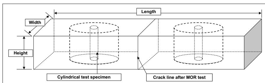
Fig. 2 Demands on a suitable test specimen, especially designed for drilling cylindrical test pieces (H = 50 mm,  $\varnothing = 50$  mm)
