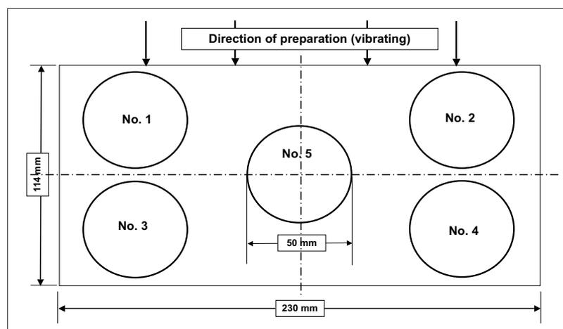
**Fig. 3 Scheme of drilling out cylindrical test specimens (H = 50 mm, Ø = 50 mm) from a vibrated test specimen shape A (230 mm x 114 mm x 64 mm)**
