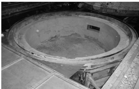
**Fig. 7 Aluminium round top melting furnace veneer lined with LPB refractory materials**
