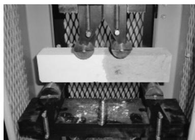
**Fig. 5** Testing equipment used to determine the bond strengths
