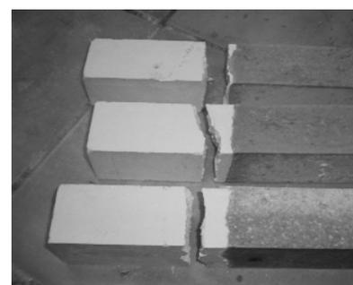
**Fig. 6** Samples after the four-point load test
