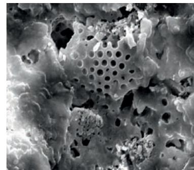
**Fig. 5** SEM image of the calcined clayey diatomite (~800 °C) for the production of absorbents; relics of diatoms are visible (NKUA)
