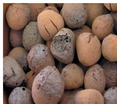
**Fig. 20** The cooled LWAs obtain a reddish colour and the characteristic porous structure (NKUA)
