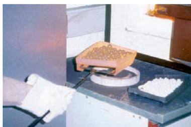
**Fig. 18** Production of LWA in a laboratory furnace
