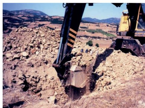
Fig. 2 Extraction of the bulk sample GRE-2 at the eastern part of the basin, the run of mine samples are wet and dark coloured
