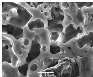
**Fig. 21** SEM images of the LWAs produced with the Greek moler; the honeycomb structure is visible (NKUA)
