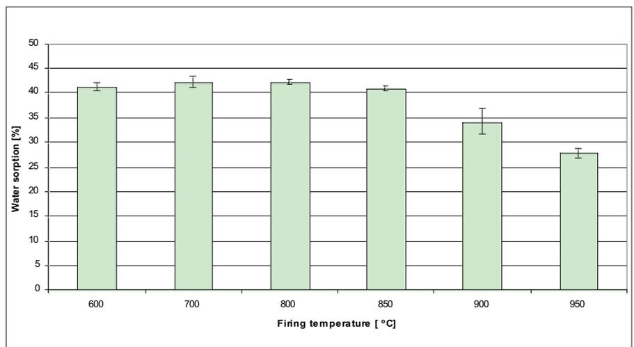
Fig. 13 Mean water sorption after 24 h immersion
