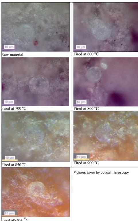
**Fig. 15** CCD images coupled with a light microscope of the diatom frustule-rich raw material fired at different temperatures
