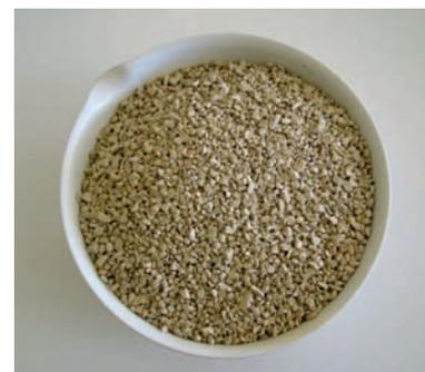
**Fig. 6** Calcined product in granules 0,3 – 1,7 mm
