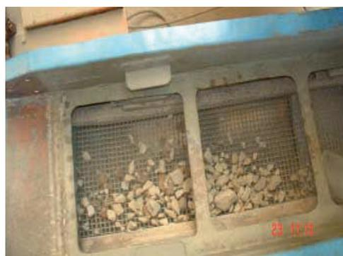
**Fig. 8** Pilot crushing – screening -10 mm
