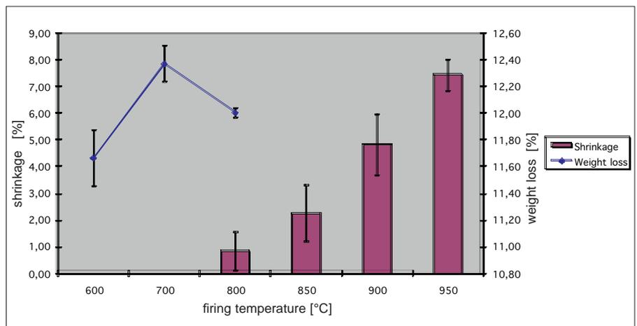
Fig. 11 Shrinkage and weight loss of the samples fired at gradient temperatures in electrical kiln (air atmosphere)
