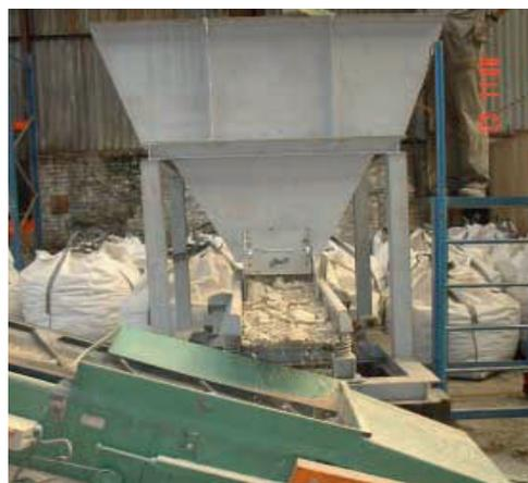
**Fig. 7** Pilot crushing – feeding device
