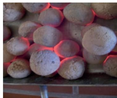
**Fig. 19** LWAs produced by the Greek clayey diatomite just pulled out from the furnace (NKUA)
