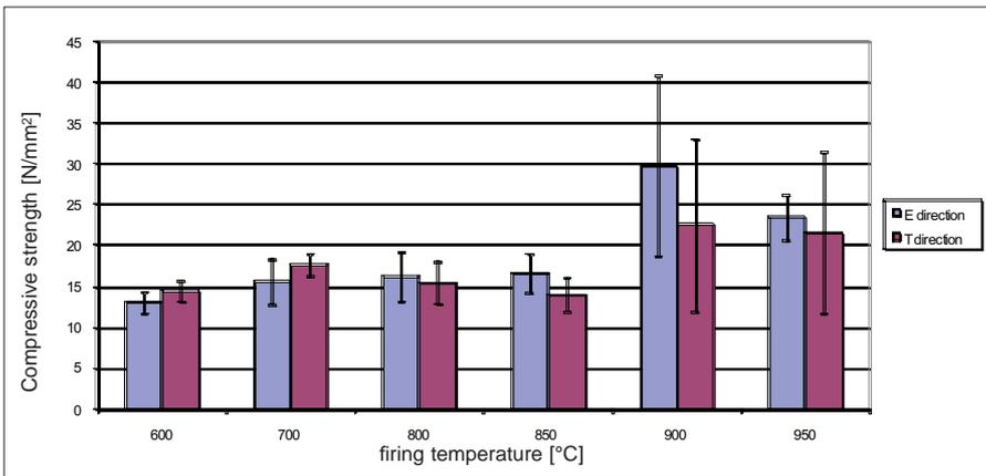
**Fig. 14** The compressive strength of the fired samples measured on 19,3-mm diameter cylinders in the extrusion direction and perpendicular to it (E and T directions respectively).
