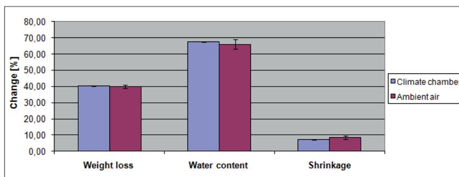
**Fig.10** Drying characterization of the extruded parallel-epiped samples (rectangular section 25 mm × 30 mm)
