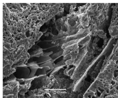
**Fig. 22** SEM images of the LWAs produced with the Greek moler; the glassy phase predominates (NKUA)
