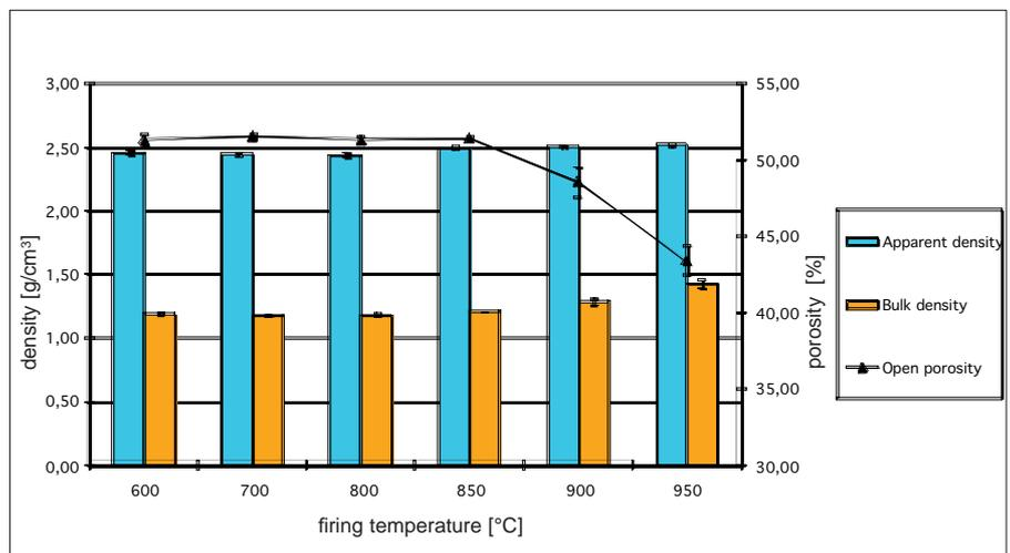
Fig. 12 Densities (bulk and apparent) and porosity of the samples fired at gradient temperatures in electrical kiln (air atmosphere). The gradient heating program used was: 20 – 600 °C, 150 °C/h; 600 – 950 °C, 200 °C/h; duration at 950 °C for 3 h; 950 – 600 °C, 200 °C/h; 600 – 500, 50 °C/h; 500 – 20 °C free
