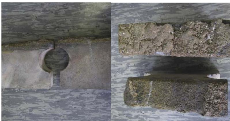
**Figs. 9 and 10 Refrax® PLUS belly bricks after 6000 h of operation**
