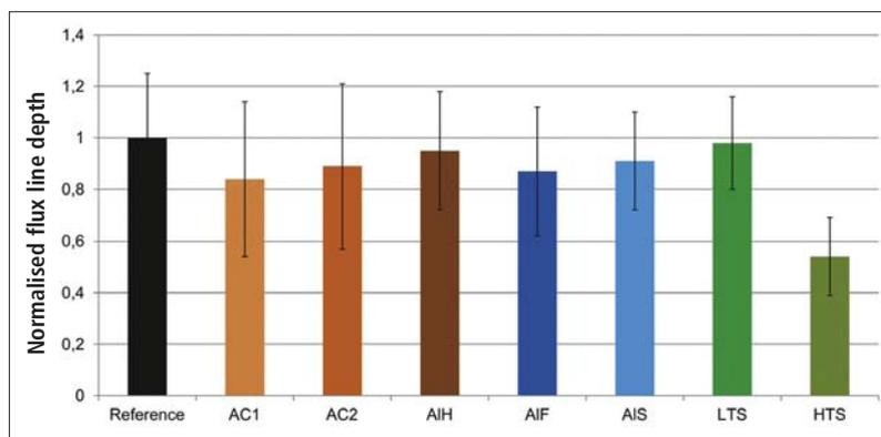
Fig. 5 Normalised flux line depth of the bricks after glass corrosion at 1550 °C after 24 h
