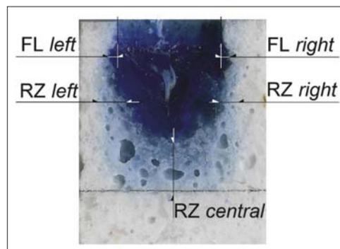
Fig. 4 Measuring of the flux line (FL) and reaction zone (RZ) at the crucibles
