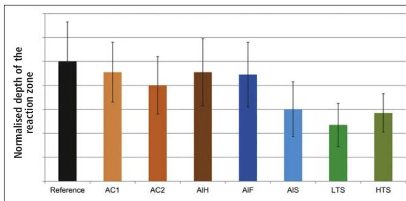
Fig. 6 Normalised thickness of the brick reaction zone after glass corrosion at 1550 °C / 24 h
