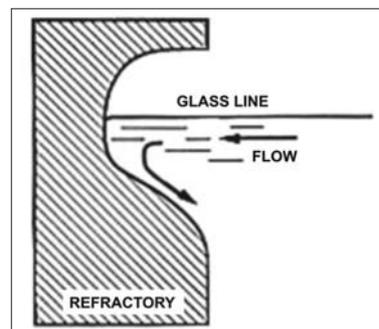
Fig. 1 Three-phase interface in a glass tank
