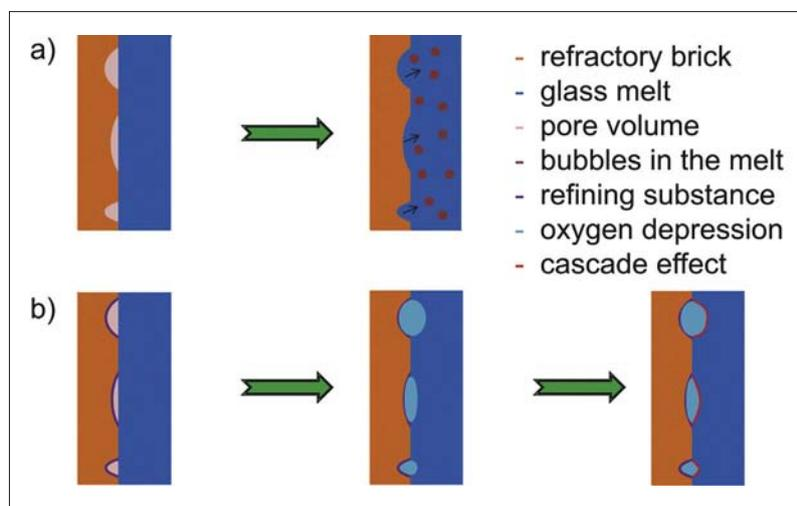
**Fig. 3** Untreated brick (a) and treated brick (b) with increasing glass surface tension (middle) and cascade effect (right)
