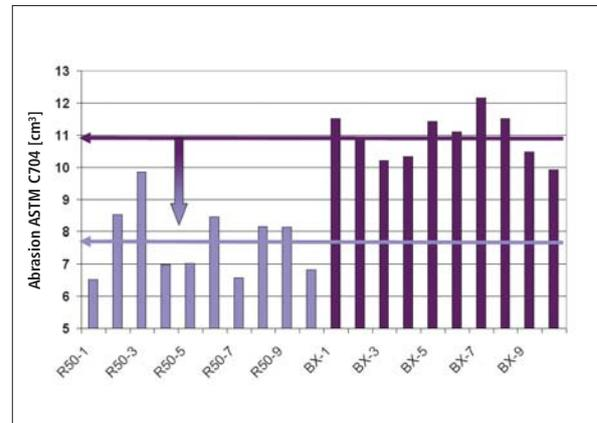
Fig. 8 Abrasion repeatability test with 10 samples of castable CC-R50 (left) and of castable CC-BX (right)
