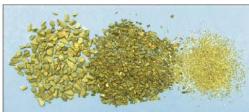
**Fig. 2 R50 aggregates (fraction 3–5, 1–3 and 0–1 mm)**
