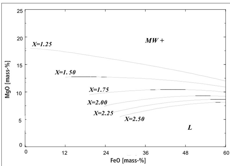
**Fig. 7** MgO saturated lines in the FeO–MgO–CaO–SiO<sub>2</sub> system as a function of the slag basicity ( $\text{CaO}/\text{SiO}_2 = X$ ), at 1600 °C and high oxygen partial pressure ( $p_{\text{O}_2} = 10^{-4.72}$  atm) [7]
