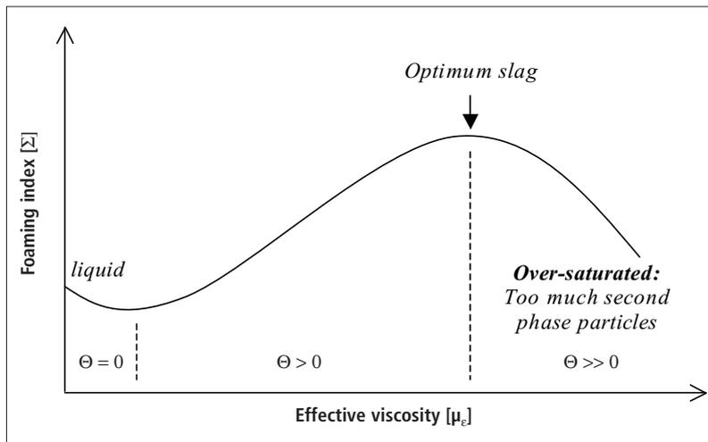
Fig. 4 The relationship between foaming index and effective viscosity [28]
