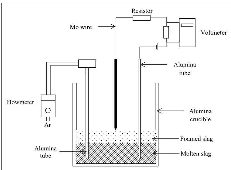
**Fig. 2** Experimental apparatus used to measure the slag height when gas is injected into the molten slag [19]
