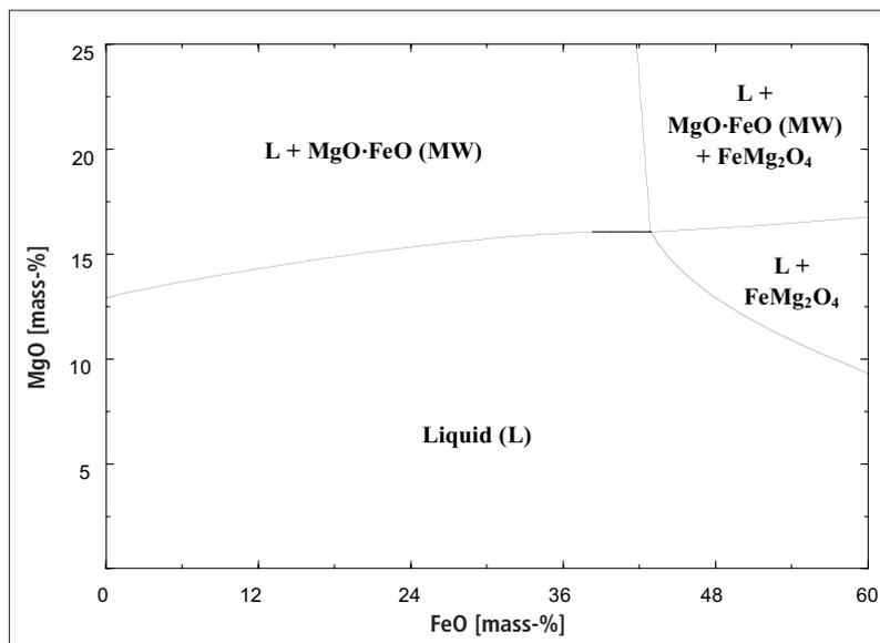
**Fig. 8** Phase diagram in the FeO–MgO–SiO<sub>2</sub>–CaO–Al<sub>2</sub>O<sub>3</sub> system for a basicity  $B_3 = 0.9$ , temperature = 1600 °C and  $pO_2 = 0.21$  atm
