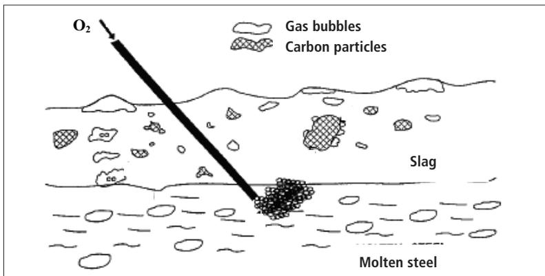
**Fig. 1** Sketch of the transformations that take place in EAF equipment during the slag foaming procedure [7]
