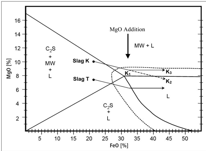
**Fig. 6** ISD diagram showing the effect of adding MgO to the path of the liquid composition [28]
