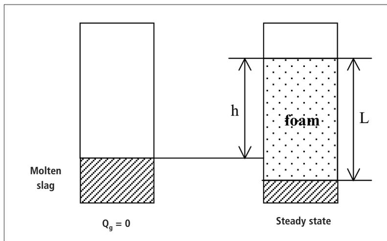
Fig. 3 Sketch of the foaming index measuring procedure [14]
