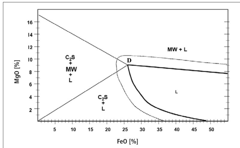
**Fig. 5** Isothermal solubility diagram (ISD) of the FeO–MgO–SiO<sub>2</sub>–CaO–Al<sub>2</sub>O<sub>3</sub> system for a basicity  $B_3$  of 2.0 and temperature = 1600 °C [28]; MW = MgO·FeO, C<sub>2</sub>S = 2 CaO·SiO<sub>2</sub>, L = liquid
