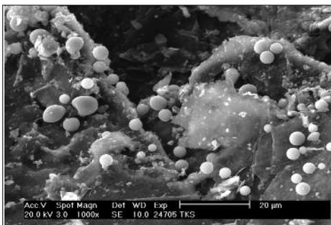
**Fig. 8** Microstructure in detail taken from the cold face; typical amounts of silica-rich aluminosilicate (spheroids), also referring to [1]
