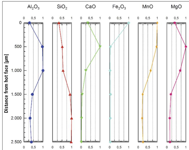
**Fig. 7** Profile of essential penetration phases from slag components into the aluminosilicate-carbon composition (normalized relative phase quantities) without consideration of the contained carbon
