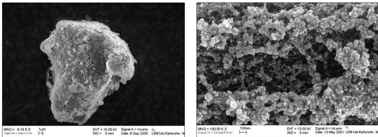
**Fig. 3** Typical, irregularly restricted grain represented the alumosilicate from "Eisenberger Klebsand", surrounded by clay particles (left side), structural construction of spherical Al-Si-gel phases of a loosely connected aggregate (right side)
