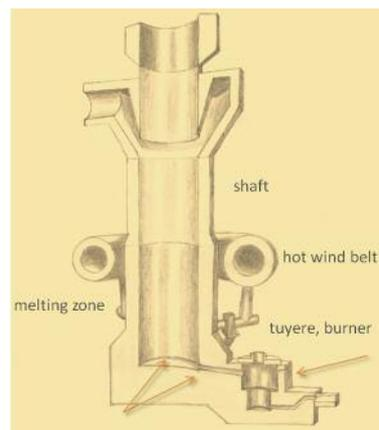
**Fig. 1** Exemplary schematic representation of a shaft furnace (after EKW, Eisenberg/DE) with focus on essential, high-efficiency refractory demands up to and above the tuyere level, furthermore peripheries (see arrows)
