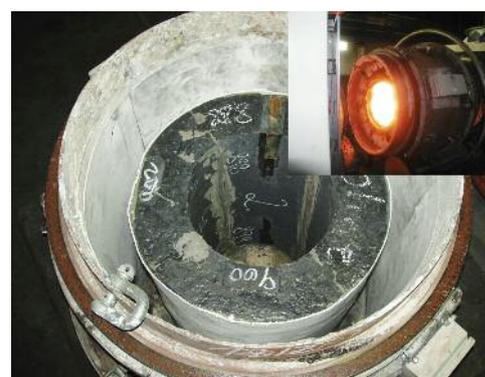
**Fig. 5** Set-up of the composites, rotary furnace experiment, conducted at *ThyssenKrupp Steel*, Duisburg/DE. The evaluated aluminosilicate-carbon composites are signed with white coloured numbers
