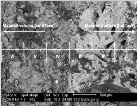
**Fig. 6** Microstructure of the reaction profile related to slag-refractory interaction
