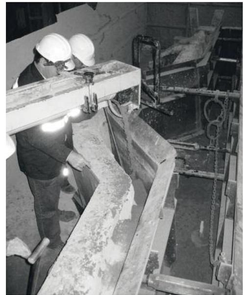
**Fig. 7** Installation of the cold setting mix at GSW Santander
