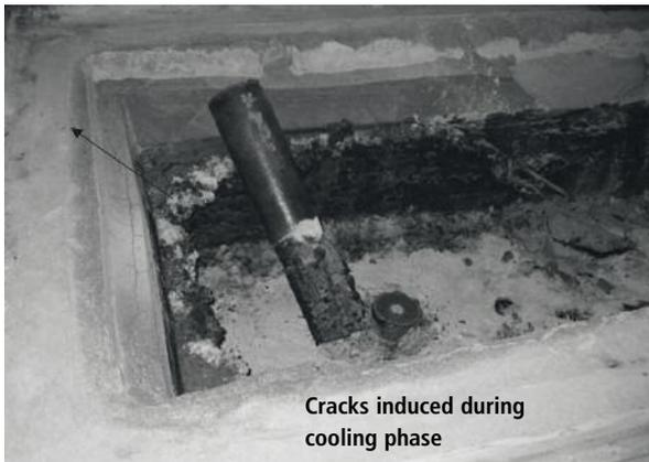
**Fig. 4** Easy deskulling after cooling down
