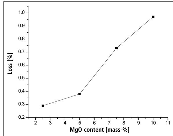
Fig. 10 Variation in corrosion resistance with MgO content for batch 3
