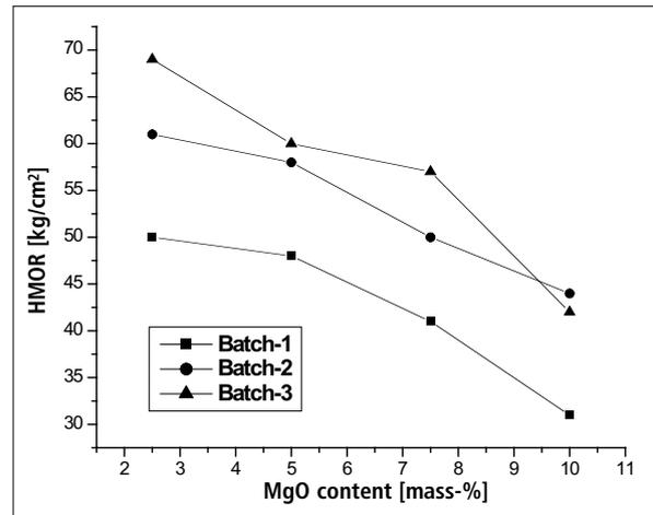
Fig. 6 Variation in hot modulus of rupture with MgO content for the sintered specimens
