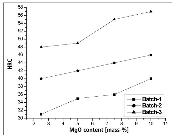
Fig. 8 Variation in hardness with MgO content for the sintered specimens
