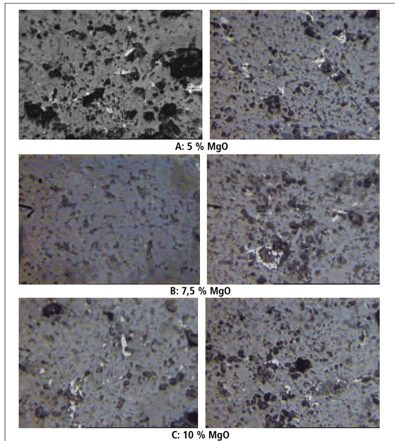
Fig. 11 Photomicrograph of the batch 3 specimens after acid etching (x 100)
