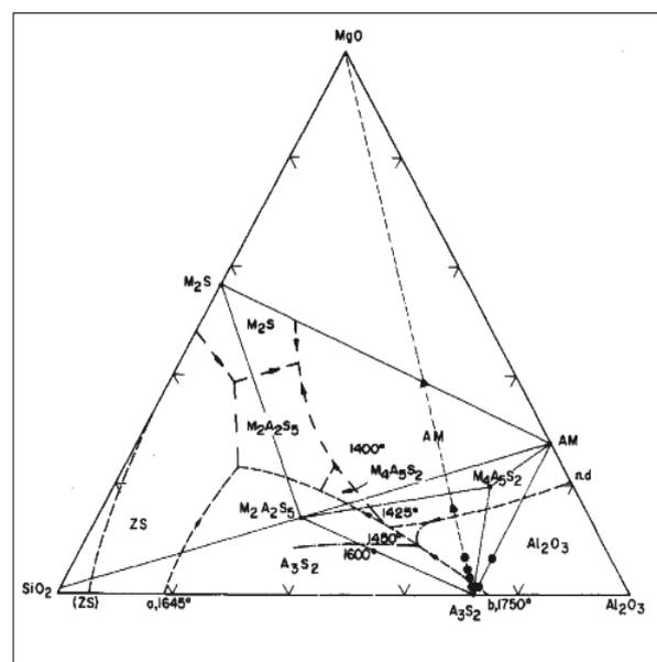
**Fig. 2** Projection of the primary volume of crystallization of ZrO<sub>2</sub> in Al<sub>2</sub>O<sub>3</sub>-MgO-SiO<sub>2</sub> ternary phase diagram
