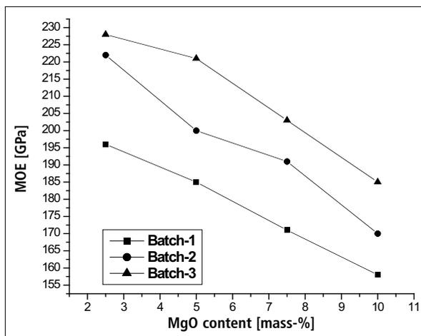
Fig. 7 Variation in modulus of elasticity with MgO content for the sintered specimens
