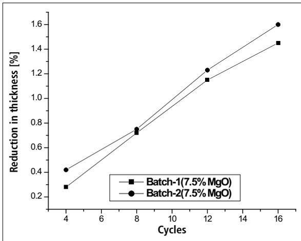
Fig. 9 Variation in abrasion resistance with number of abrasion cycles
