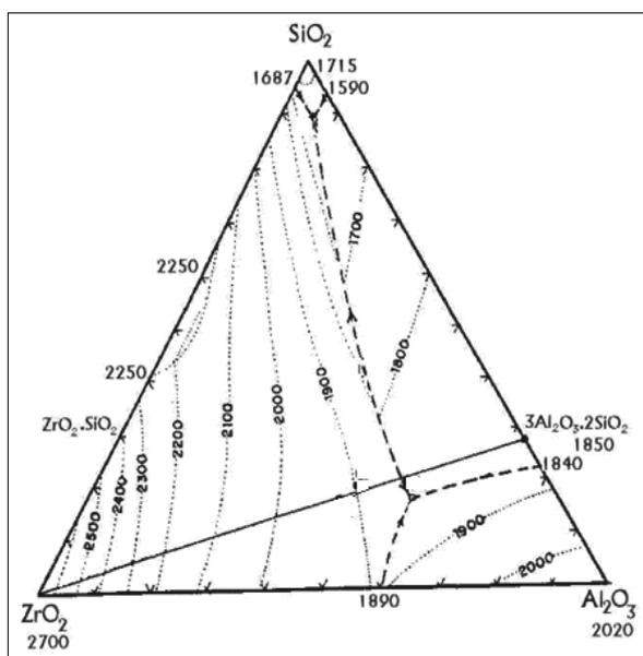
**Fig. 1** Phase equilibrium diagram of ZrO<sub>2</sub>-Al<sub>2</sub>O<sub>3</sub>-SiO<sub>2</sub> for liquidus projection [°C]
