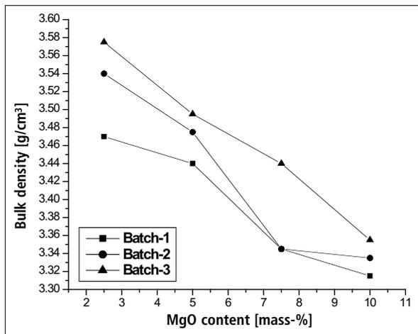
Fig. 3 Variation in bulk density with MgO content for the sintered specimens
