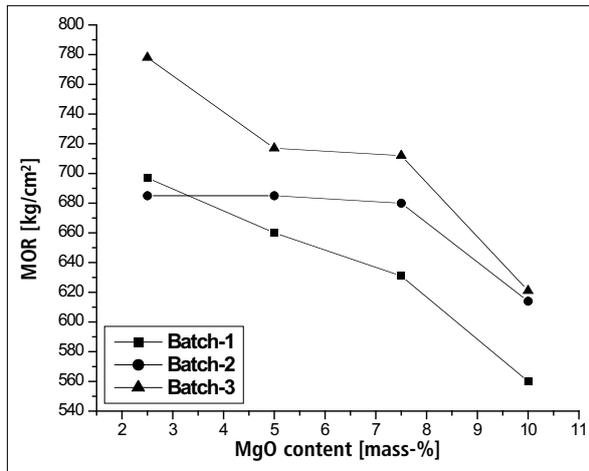
Fig. 5 Variation in modulus of rupture with MgO content for the sintered specimens
