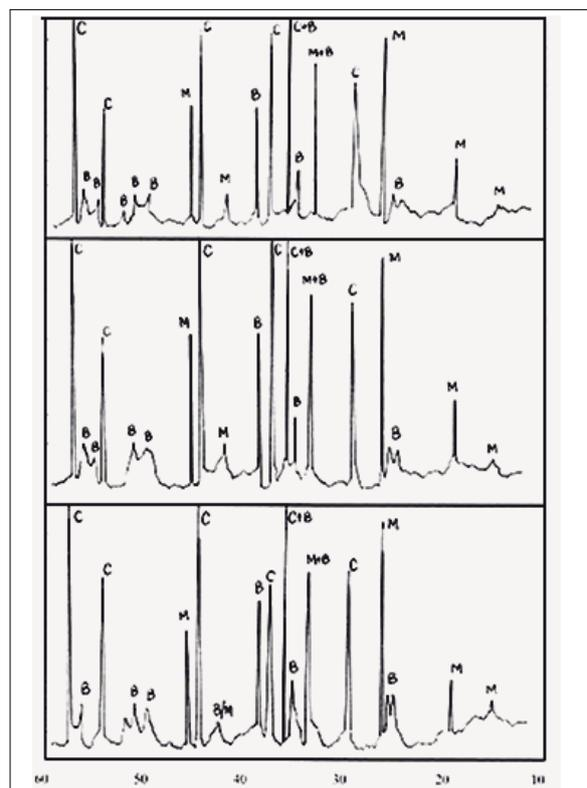
**Fig. 13** XRD diagramme of the sintered specimens of batch 3 with MgO (top to bottom: 5 % MgO, 7,5 % MgO and 10 % MgO) additive (B = ZrO<sub>2</sub>(m), M = mullite, C = corundum, S = spinel)
