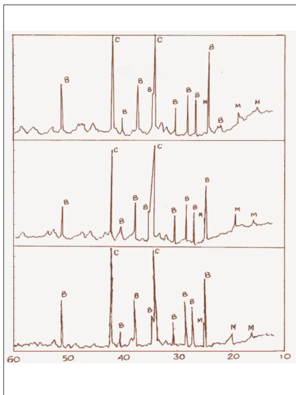
**Fig. 12** XRD diagramme of the sintered specimens (top to bottom: batch 3, batch 2, batch 1) without additive (B = ZrO<sub>2</sub>(m), M = mullite, C = corundum)
