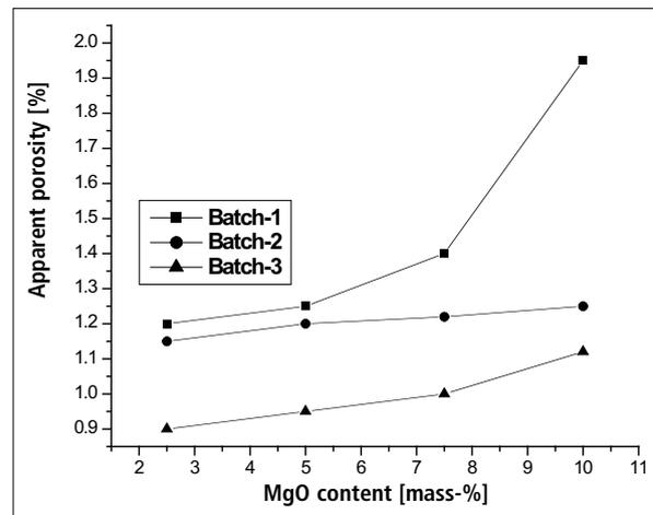
Fig. 4 Variation in apparent porosity with MgO content for the sintered specimens
