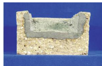
Fig. 8 Cup test failure
