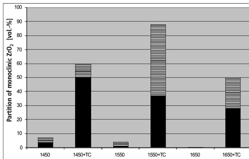
**Fig. 8** Partition of monoclinic  $\text{ZrO}_2$  as determined by EBSD in dependence on the sintering temperature (6 h) and an additional thermal cycling between room temperature and 1300 °C (dilatometer)
