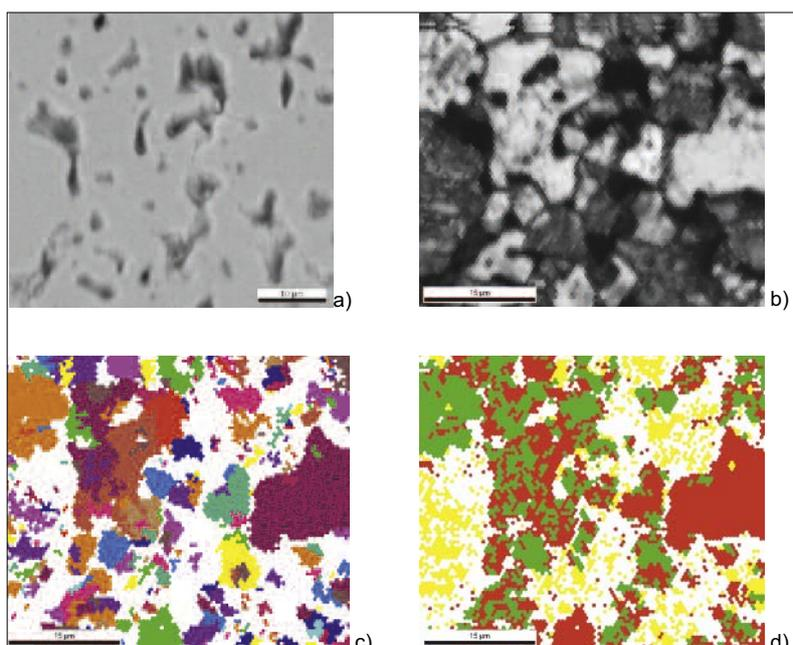
**Fig. 5** Sample PSZ, sintering temperature 1550 °C and an additional thermal cycling between room temperature and 1300 °C (dilatometer)
