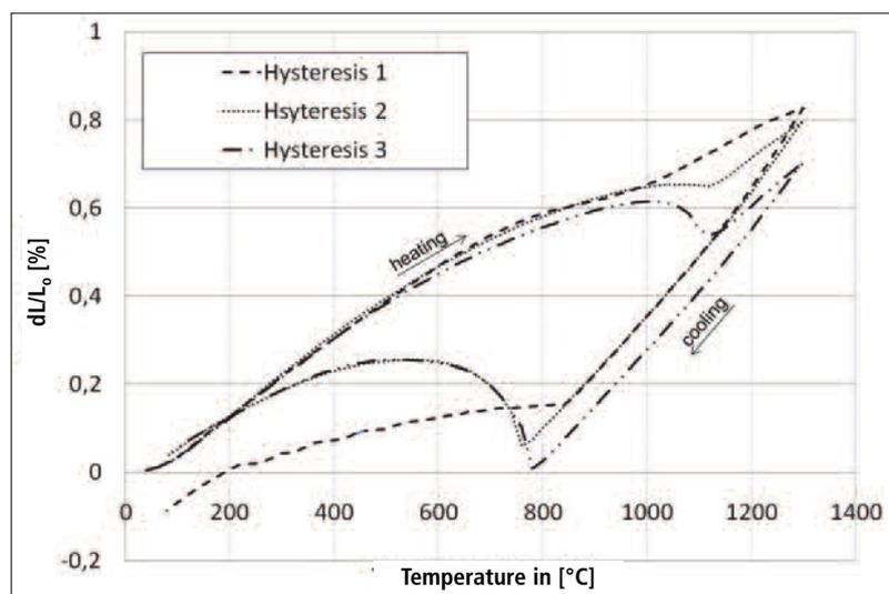
**Fig. 3** Thermal expansion curves of the Mg-PSZ ceramic sintered at 1450 °C
