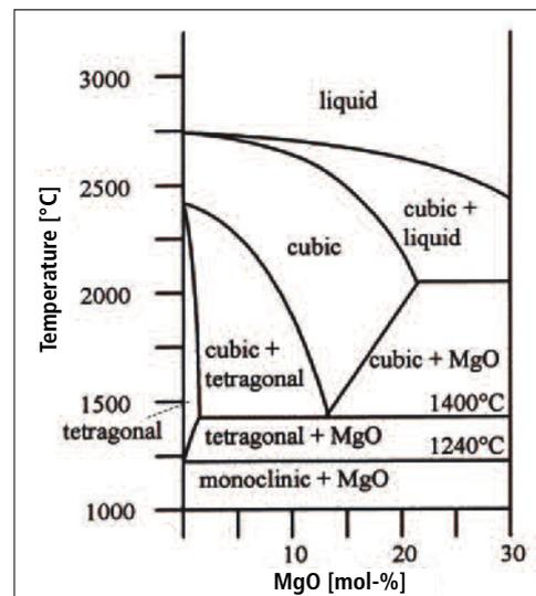
Fig. 1 Phase diagram of partly MgO-stabilized  $\text{ZrO}_2$  [15]
