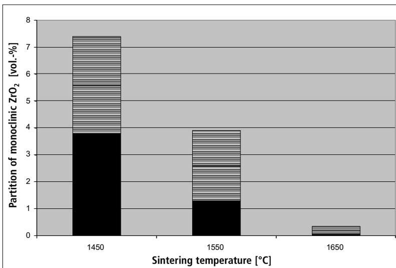
**Fig. 7** Partition of monoclinic ZrO<sub>2</sub> as determined by EBSD in dependence on the sintering temperature, and corresponding standard deviations
