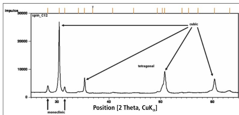
**Fig. 9** Typical XRD spectrum of PSZ in the small angle range with overlapping of the cubic and tetragonal peaks
