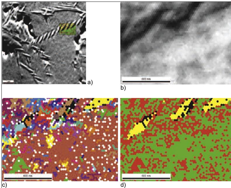
**Fig. 6** Sample PSZ, sintering temperature 1650 °C; SE image and EBSD analysis of an area with monoclinic lenses
