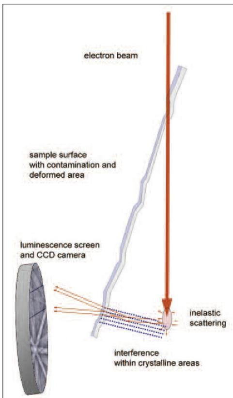
**Fig. 2** Principle of electron backscatter diffraction (EBSD)
