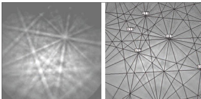
**Fig. 4** Typical EBSP of cubic  $ZrO_2$  and corresponding indexing
