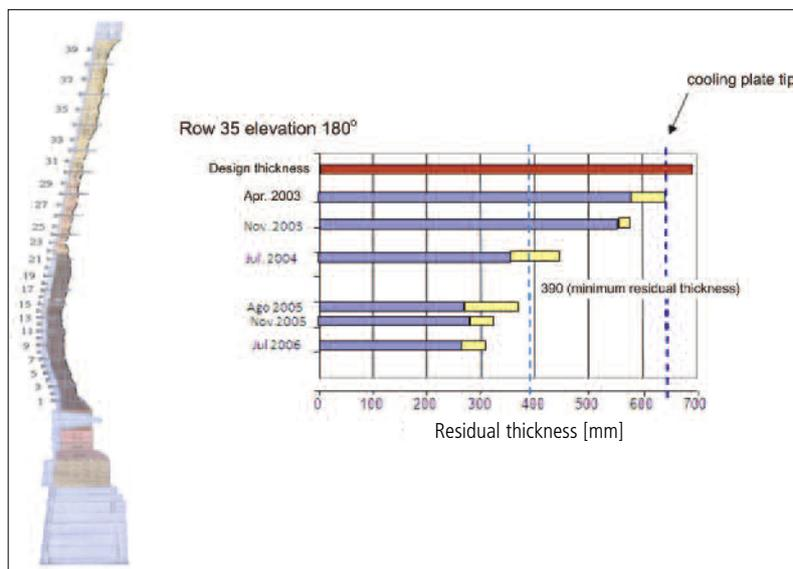
**Fig. 4** Wear profile behaviour of refractory lining of upper stack at row 35 cooling plates elevation (ref.: 2003 – 2006 time frame)
