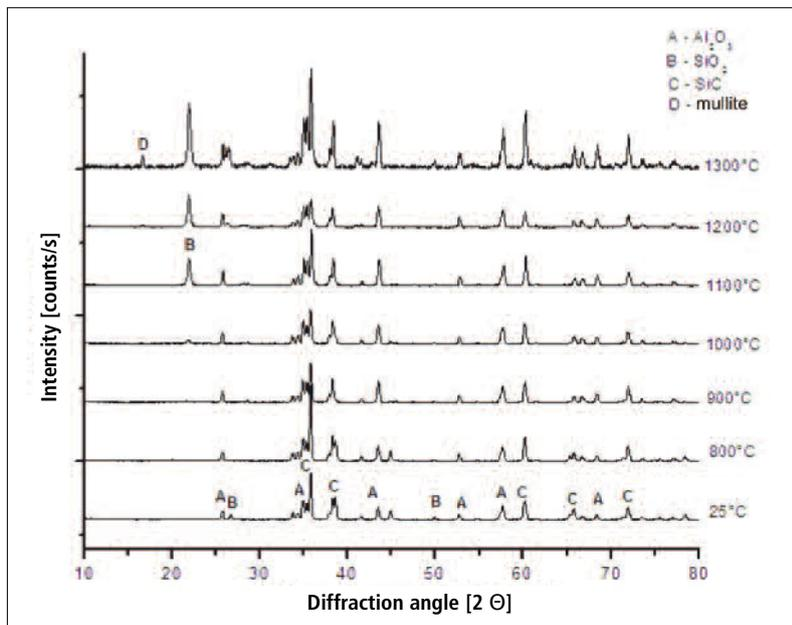
**Fig. 7** XRD of castable super fine fraction mixture used in lower and mid stacks with 12 mass-% binder and 1 mass-% setting accelerator after heat treatment
