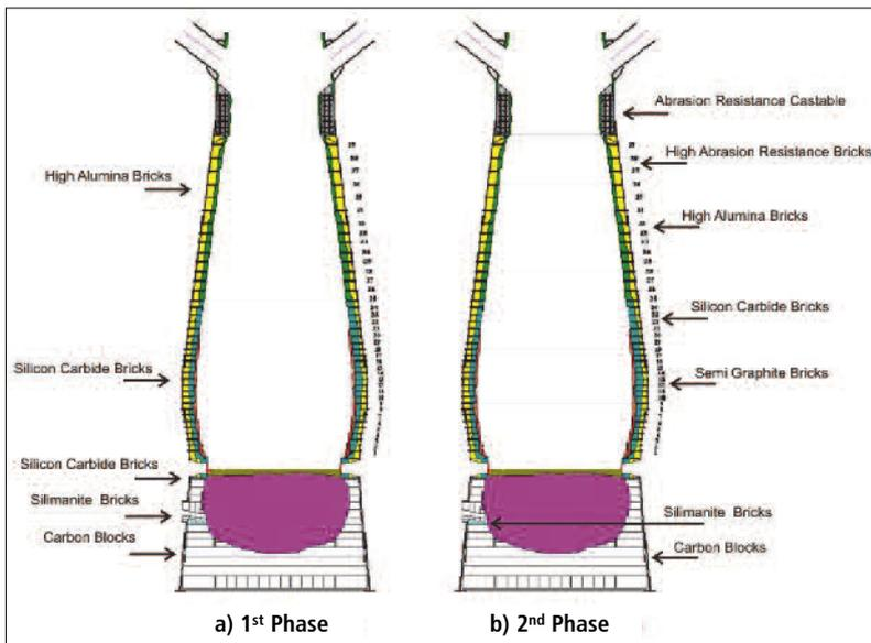
Fig. 3 Refractory lining design before and after 2000 partial repair
