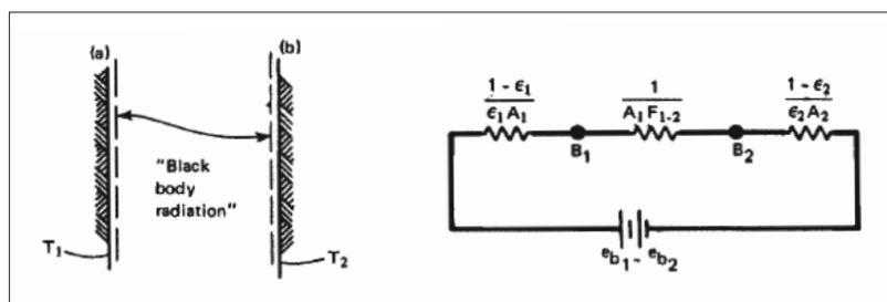
**Fig. 5 The electrical circuit analogy for radiation between two grey plates**
