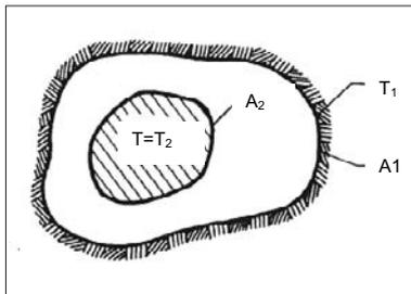
**Fig. 6** Heat transfer between an enclosed body and the body surrounding it
