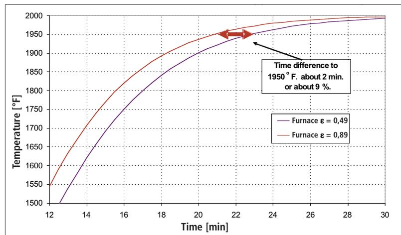
**Fig. 8** Heat-up rates for steel blocks based on theoretical calculations for radiant heat transfer only (1500 °F and above)
