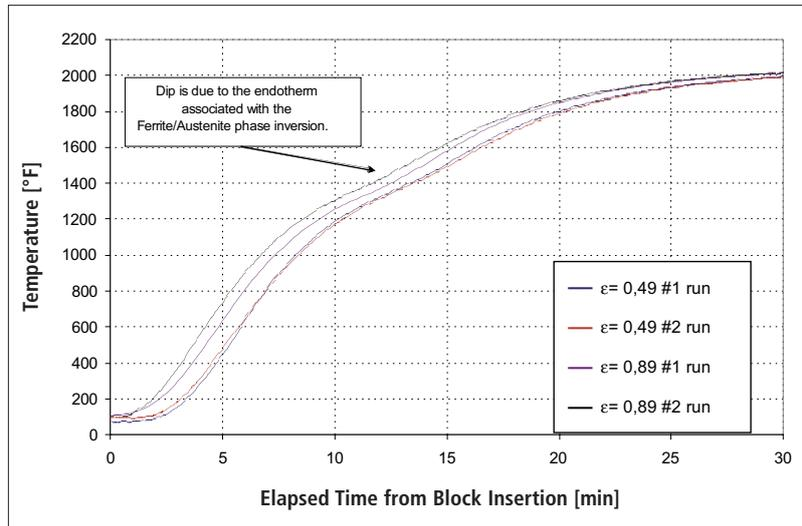
Fig. 9 Experimental steel block heat-up rates
