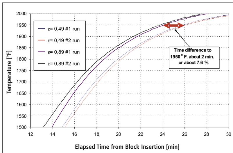
Fig. 10 Experimental steel block heat-up rates (1500 °F and above)
