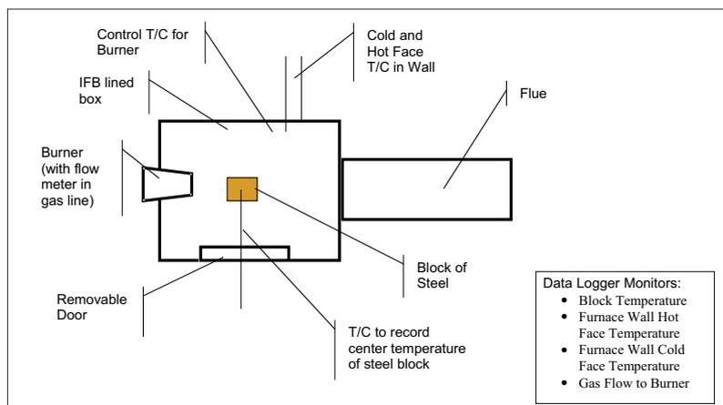
Fig. 1 Scheme of experimental set-up
