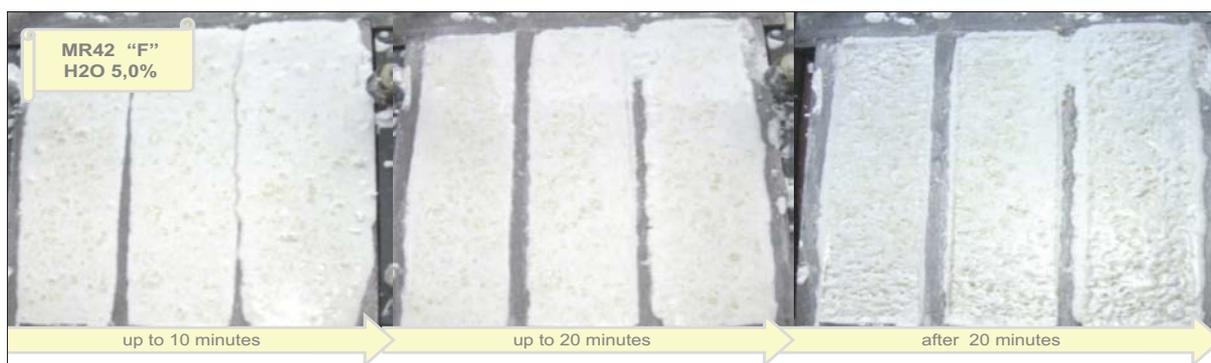
**Fig. 2** The product was cast directly into the mould (flowability value about 190 mm); within the first 10 min the consistency of the castable changed (small holes were visible on the surface); after about 20 min the surface of the castable became very rough with "cheese"-like holes within the complete structure. Such behaviour may be difficult to control on the job site during the installation of the product
