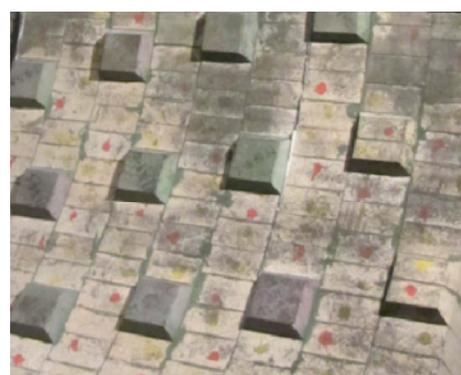
Fig. 2 Hump area in the inlet zone of a rotary kiln
