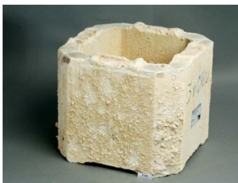
**Fig. 2** The spinel-bonded magnesia brick (RUBINAL ESP) after 3 years application
