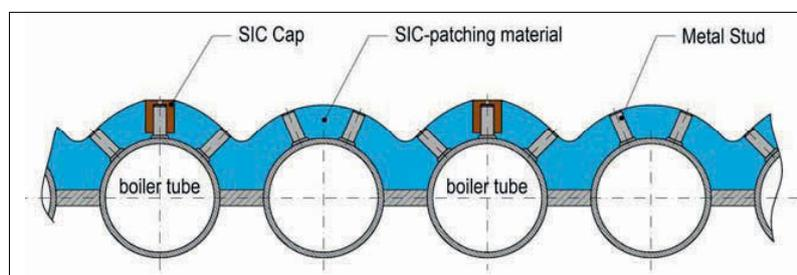
**Fig. 11** Boiler tube coated with phosphate bonded SiC patching material
