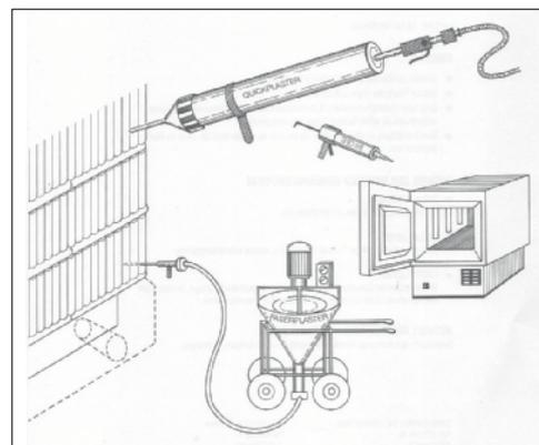
**Fig. 9** Maintenance with plastic fibre-mastic
