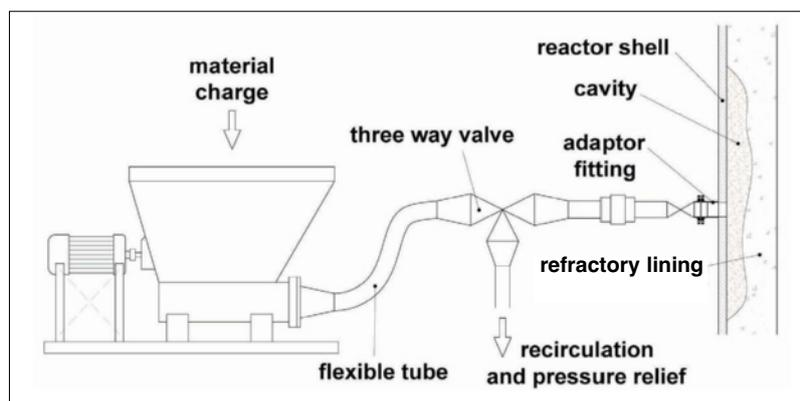
**Fig. 8** Principle outline of high pressure injection (muxing)
