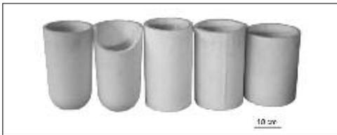
**Fig. 7** Refractory crucibles for heat-proof alloys induction melting
