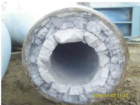
**Fig. 3** Transfer line showing hot face and insulation layers
