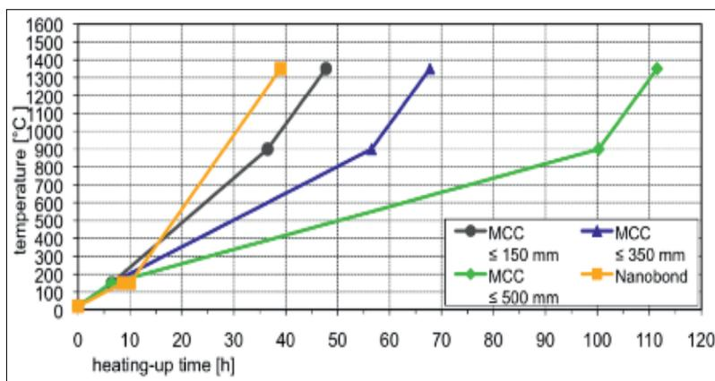
**Fig. 1** Heating-up procedure of different medium cement castables samples compared to Nanobond
