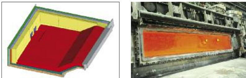
**Fig. 4 a–b** Melting furnace no. 6 at TRIMET (Essen): relined areas of the aluminium melting furnace (red colour) and a view into the furnace after heating up and during sintering with liquid metal
