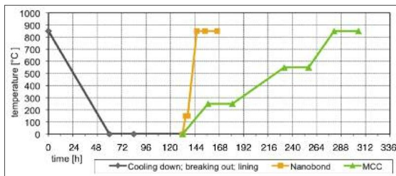
**Fig. 5 Total time schedule for relining the aluminium melting furnace: Nanobond and medium cement castable (MCC)**
