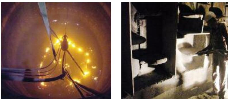
**Figs. 3 a–b** Hot robotic jetcasting (l.) and cold manual jetcasting from working platform (r.)
