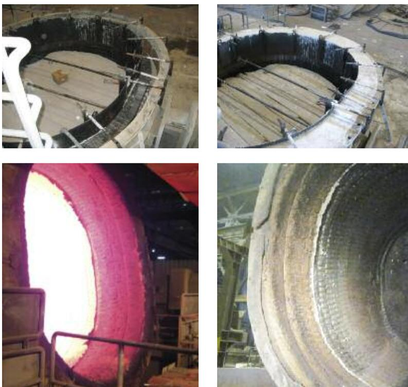
**Figs. 2 a–e** Steel ladle before and after casting the upper free board with Nanobond (top) and after 16 (lower left) and after 65 batches (lower right)
