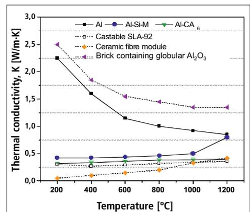
**Fig. 3** Thermal conductivity of the sintered foamed ceramics (Al, Al-Si-M and Al-CA<sub>6</sub>) and commercial insulating materials (some results were adapted from reference [13])
