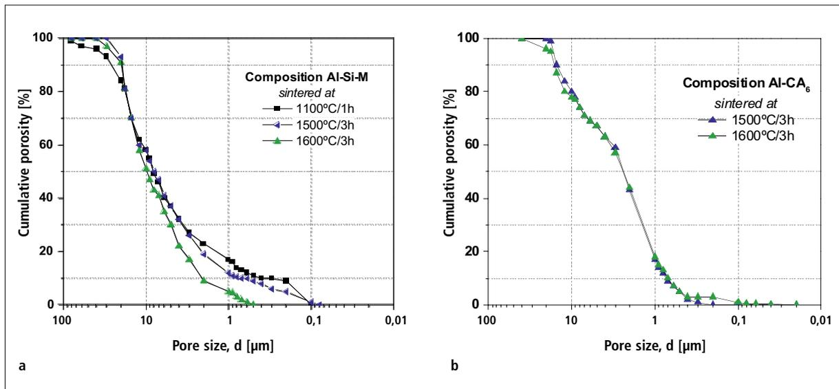
**Fig. 4** Thermal treatment effect on the pore size distribution of (a) Al-Si-M and (b) Al-CA<sub>6</sub> foamed ceramics
