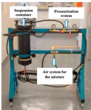
**Fig. 1** Foaming equipment developed by Salvini et al. [11]
