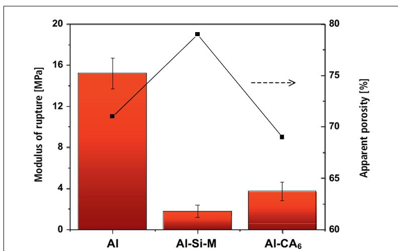
**Fig. 5** Splitting tensile resistance and apparent porosity of the porous ceramics after sintering (firing temperatures: Al = 1500 °C/5 h, Al-Si-M = 1100 °C/1h, and Al-CA<sub>6</sub> = 1500 °C/3 h)
