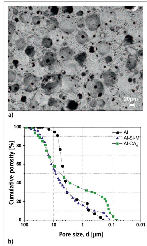
**Fig. 2** a) Cross section area of the Al sample sintered at 1500 °C/5 h, and (b) pore size distribution of the porous ceramics after firing at 1100 °C/1 h (Al-Si-M), 1500 °C/3 h (Al-CA<sub>6</sub>) and 1500 °C/5 h (Al)
