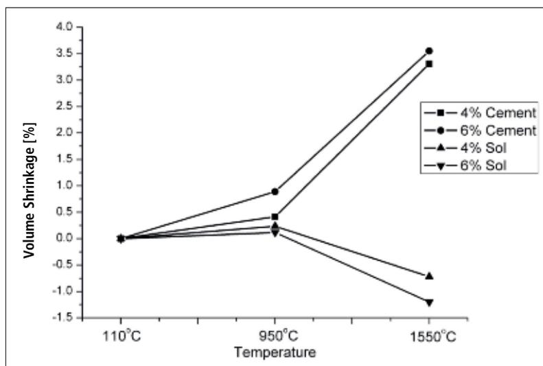
Fig. 4 Variation of volume shrinkage against temperature
