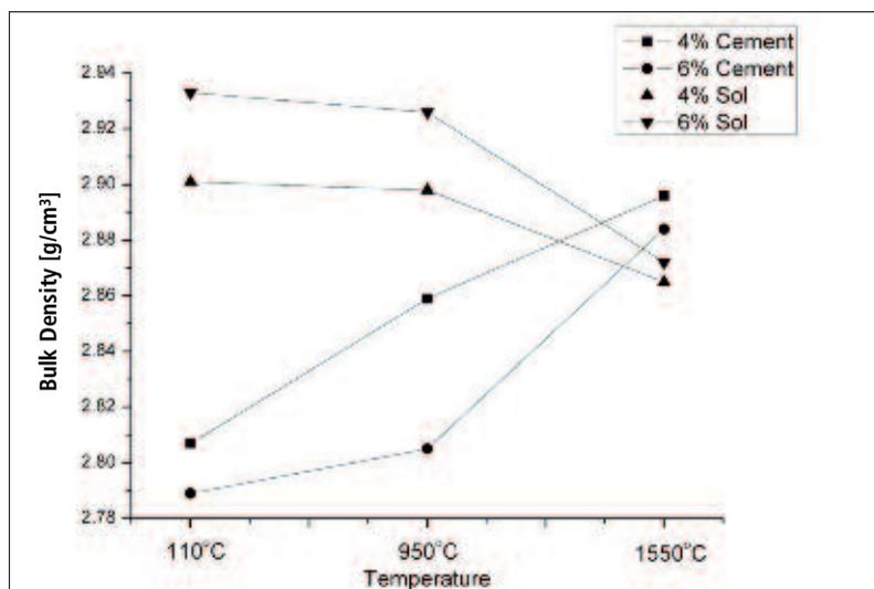
Fig. 3 Variation of bulk density against temperature
