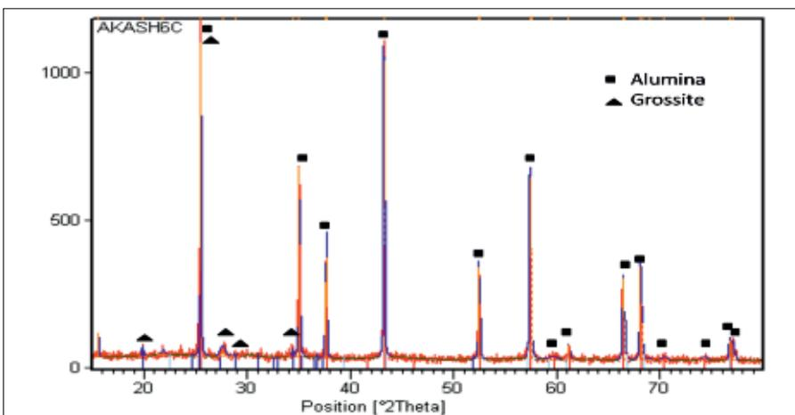
**Fig. 2b** XRD plot of 6 mass-% high alumina cement-based castables fired at 1550 °C
