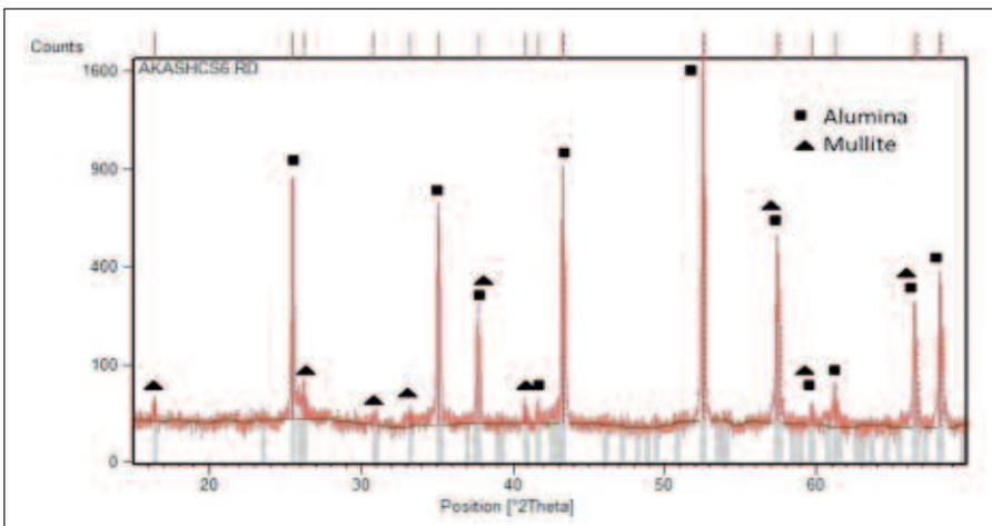
**Fig. 2a** XRD plot of 6 mass-% silica sol-based castables fired at 1550 °C
