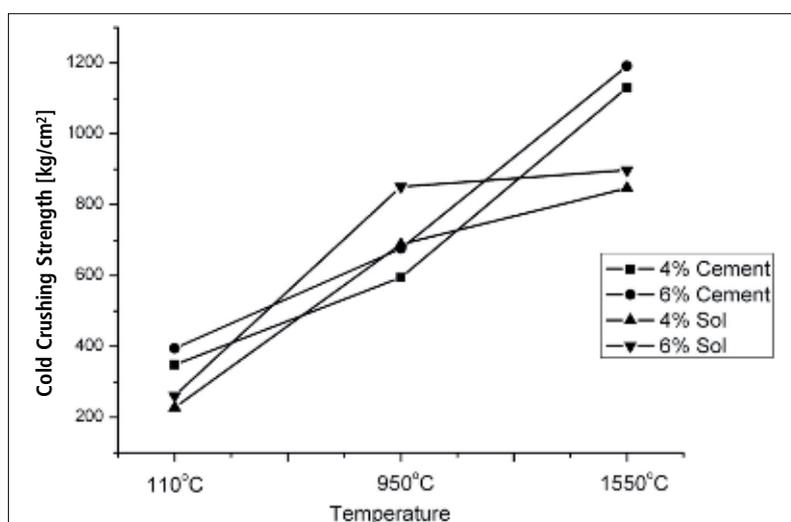
Fig. 5 Variation of cold crushing strength against temperature
