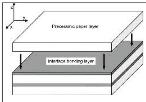
**Fig. 1 Stacking of preceramic papers for the fabrication of multilayer refractories**
