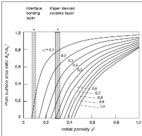
**Fig. 6** Pore surface area reduction calculated for  $\beta = 0,77$  (e.g. P-Z) for different values of degree of interface reaction versus initial porosity
