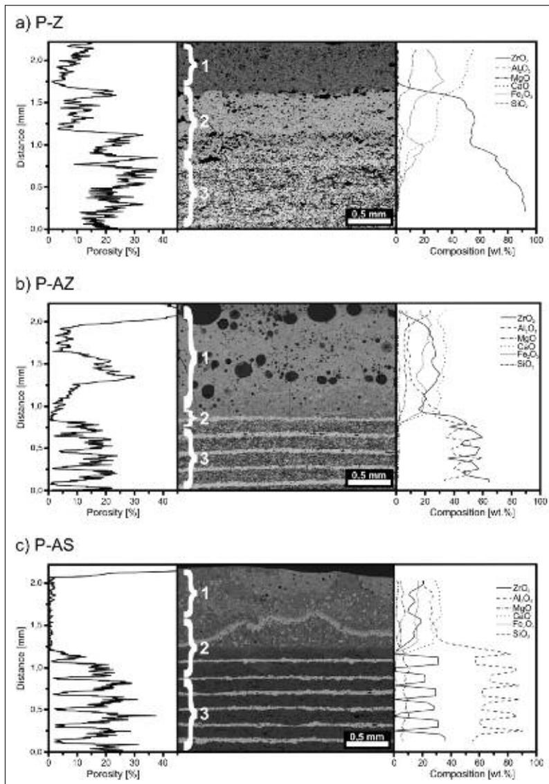
**Fig. 3 a–c** Porosity, slag infiltration behavior and element distribution of multilayer laminates derived from preceramic papers P-Z (a), P-AZ (b), and P-AS (c); microstructure of the laminates shows a slag region (1), a corrosion reaction zone (2), and the unreacted laminate material (3)
