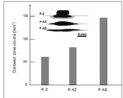
**Fig. 4** Corroded volume and slag infiltration profiles of the preceramic paper derived multilayer laminates. Slag and corroded area are drawn in black, infiltrated and partially corroded area is gray; horizontal lines represent the laminate surface
