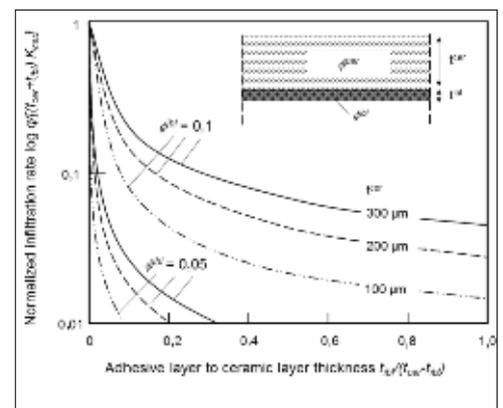
**Fig. 5** Normalized flow rate calculated for different values of initial porosity of interface bonding layer (ibl), e.g.  $\phi^{ibl} = 0,1$  and  $0,05$ , versus ibl-thickness
