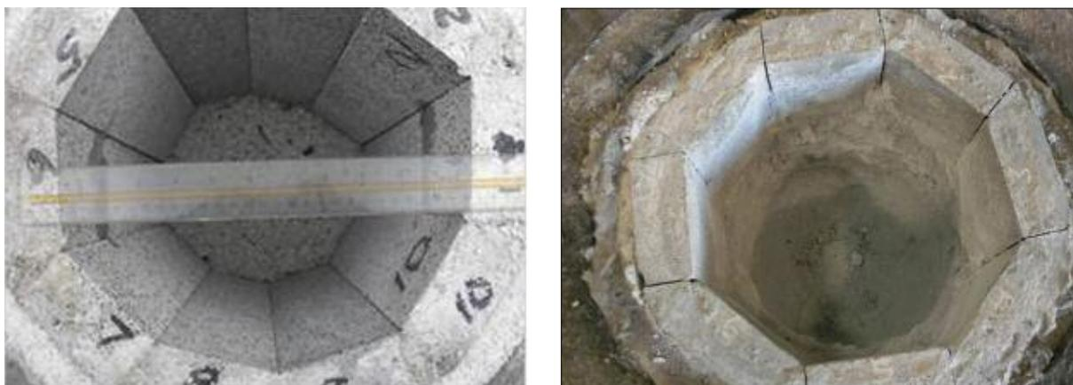
**Fig. 8** Rotary furnace simulation test system lining (a) before and (b) after testing
