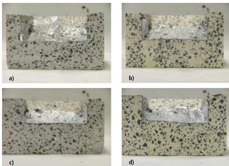
**Fig. 5** Aluminum cup penetration testing performed in 7075 aluminum alloy: a) shot sample pre-fired at 871 °C, b) shot sample pre-fired at 1260 °C, c) cast sample pre-fired at 871 °C, d) cast sample pre-fired at 1260 °C
