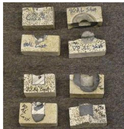
**Fig. 4** Refractory samples following *Alcoa* standardized cup testing
