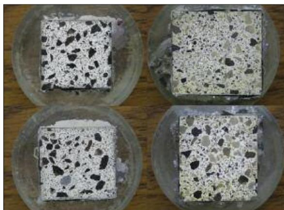
**Fig. 3** Sectioned immersion test samples of developed refractories for aluminum
