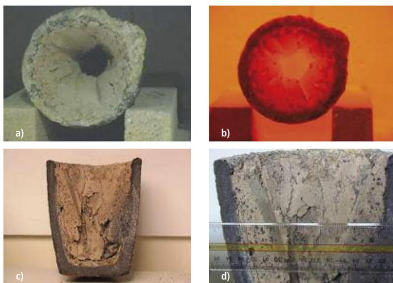
**Fig. 6** A crucible containing solidified aluminum/dross/flux: a) was heated and veneered with repair material, b) before being cooled and sectioned, c) evaluation of the coating after cooling showed good adhesion of repair material to the degraded crucible wall d)
