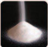
The MRA, MEGR & MEGE family of Sized Magnesium Oxides, is specifically designed for Refractory and Ceramics Industries to enhance the mechanical & thermal properties of shaped refractories and ceramic applications, among others. For these products, we only use our world's reputed raw materials that come from synthetic high purity process.
