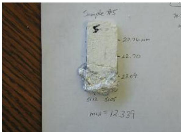
**Fig. 2** Static immersion test sample of initially developed aluminum refractory
