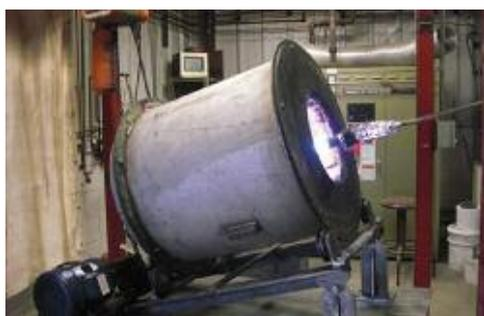
**Fig. 7** Rotary furnace simulation test system built at MINTEQ
