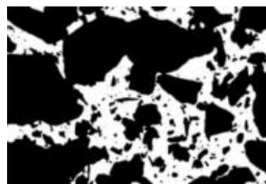
Fig. 7 Photomicrograph of Tamil Nadu graphite (plane polar)
