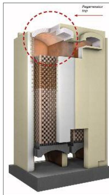
**Fig. 1** Regenerator chamber with checker work (copyright RHI AG)
