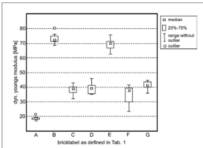
**Fig. 3** Box plot for the dynamic Young's modulus derived from impulse excitation vibration technique. The results are shown for the six different refractory materials
