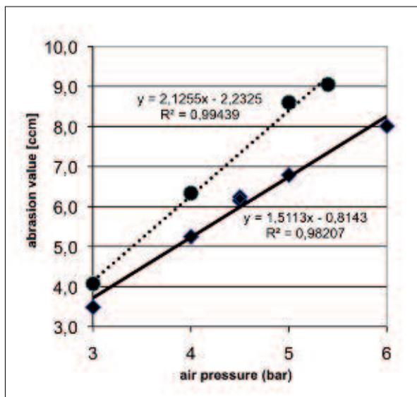
**Fig. 1** Dependence of volume loss [cm<sup>3</sup>] and air pressure [bar] on borosilicate glass plates. The results are derived in two independent laboratories; the different signatures measurements in two different laboratories
