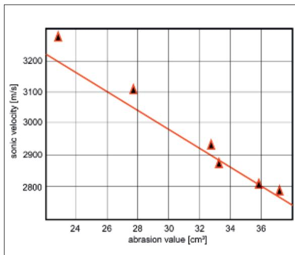
**Fig. 4** Linear dependence of the abrasion loss to the sonic velocity for sample A
