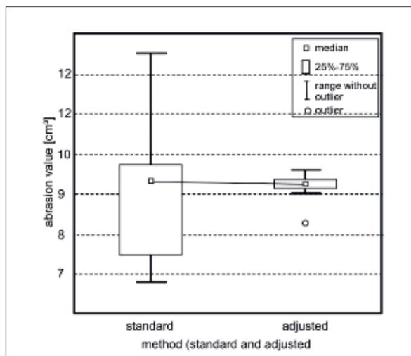
**Fig. 6** Box plot for all standard glass sample measurements. The standard deviation can be significantly reduced if the air pressure is adjusted
