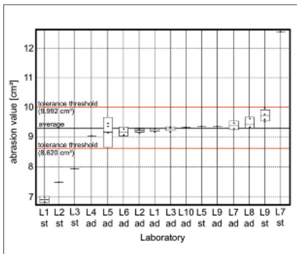
**Fig. 5** Evaluation of the precision for the standard glass samples. The figure shows results for a fixed air pressure (st) and adjusted air pressure (ad). All values derived after adjustment fall within the tolerance threshold
