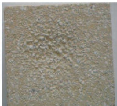
**Fig. 6** Silica sample with apparent porosity of 21 % after the abrasion resistance test, volume of removed material  $V = 5,8 \text{ cm}^3$
