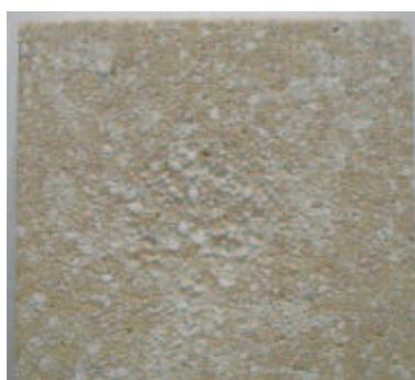
**Fig. 7** Silica sample with AP = 13 % after the abrasion resistance test, volume of removed material  $V = 2,8 \text{ cm}^3$
